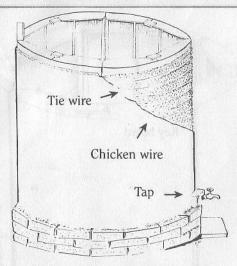
Wrap the chicken wire around the formwork. This is followed by 3-4 mm wire about 20 or 30 mm apart from each other. The tank is then plastered with mortar — one part cement to two parts of sand. The total thickness of the tank wall should not be more then 30 mm.
