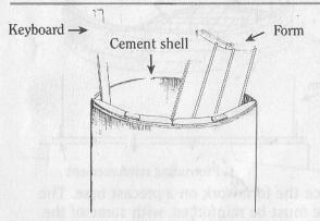
The formwork can be taken out after 24 hours. The keyboard is pulled out first. The inside of the tank is then plastered with the same mixture as the outside.
