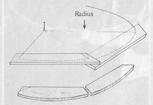
Place two boards on the edge of the circle, then draw another circle on the boards (see dotted line). Cut the boards along the dotted line. Make more cut boards to complete the circle.
