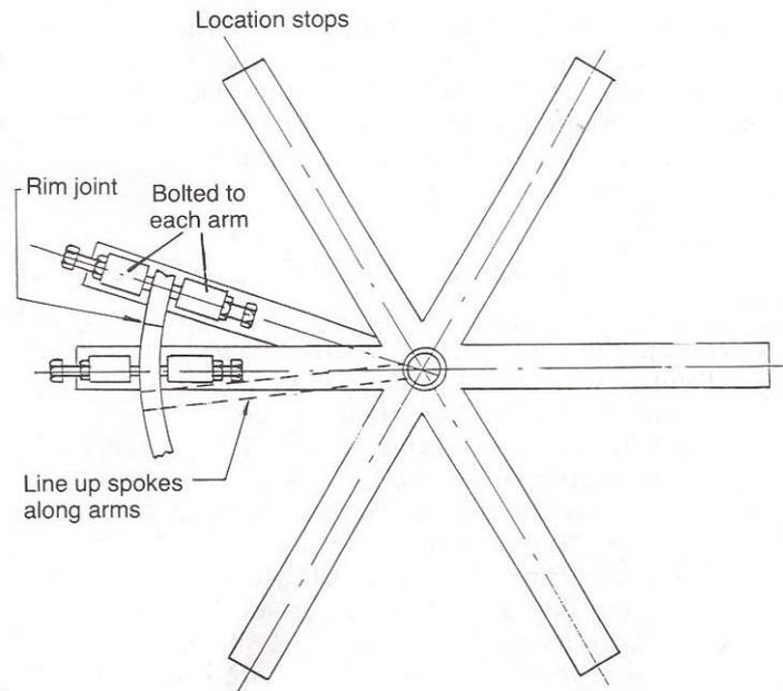
Figure 2: The assembly jig used for the construction of bicycle-type wheels.
