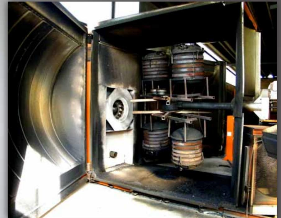
The Hippo roller mould is filled with LLDPE powder & then moved into the oven while rotating in all directions.
