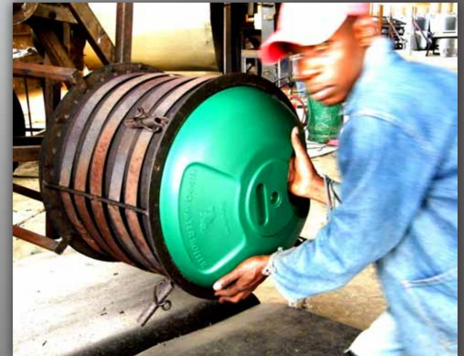
After being heated in the oven the moulds are then cooled while still rotating, after which the completed drum is removed.
