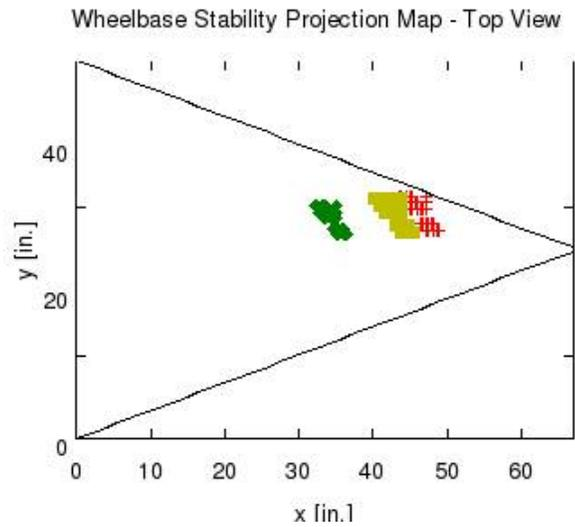
Figure 29: Projection of CG acceleration onto wheelbase in an uneven right-hand turn. Red, yellow and green points represent cargoes of 0, 40 and 250 lbs., respectively.
