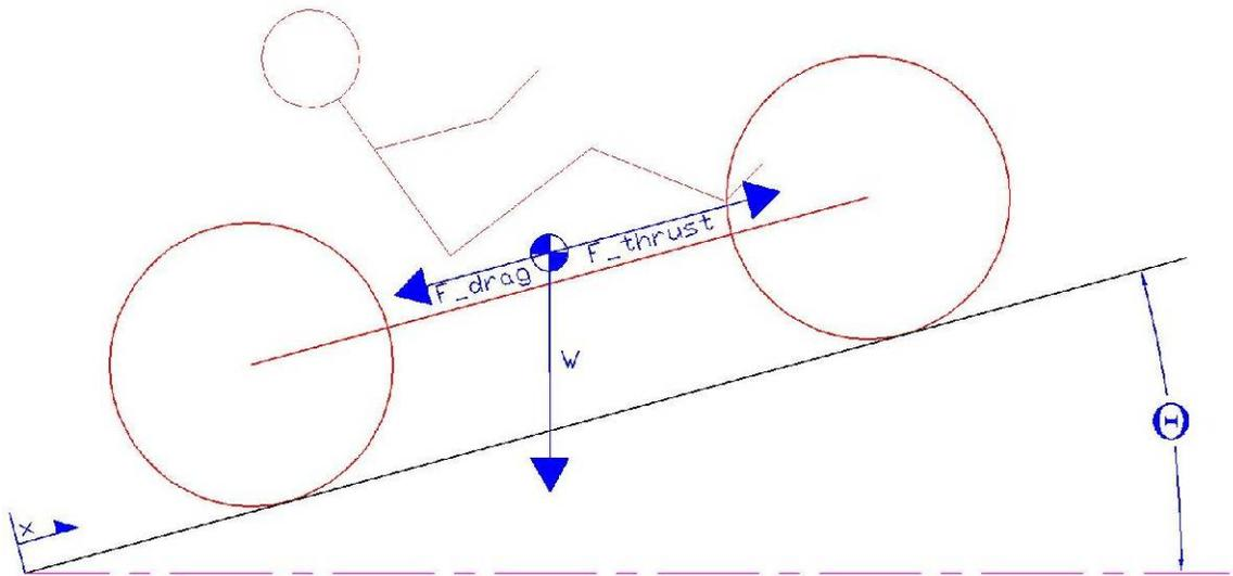
Figure 25: Simple free-body diagram for initial simulations.
