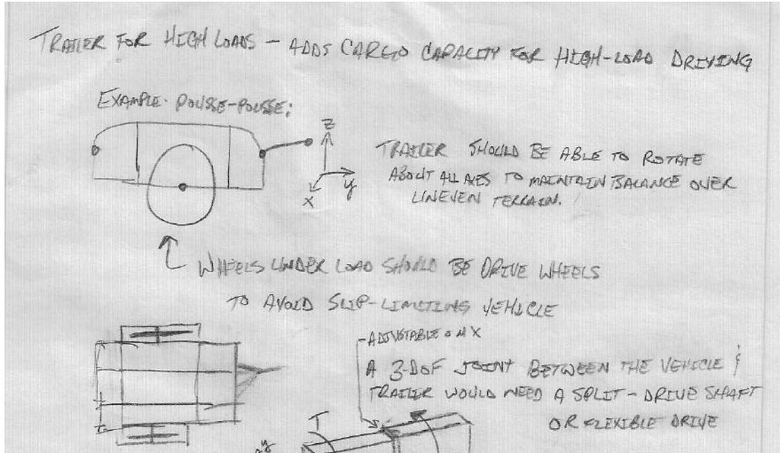
Figure 20: High-load trailer similar to Cameroonian pousse-pousse.
