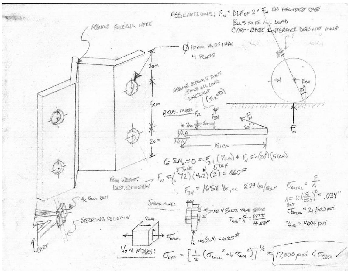
Figure 31: Example of bolt stress calculations for removable interface.
