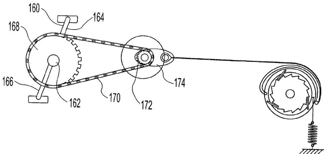
Figure 16: Beale's mechanical CVT, as shown in US Patent 7,011,322 B2.
