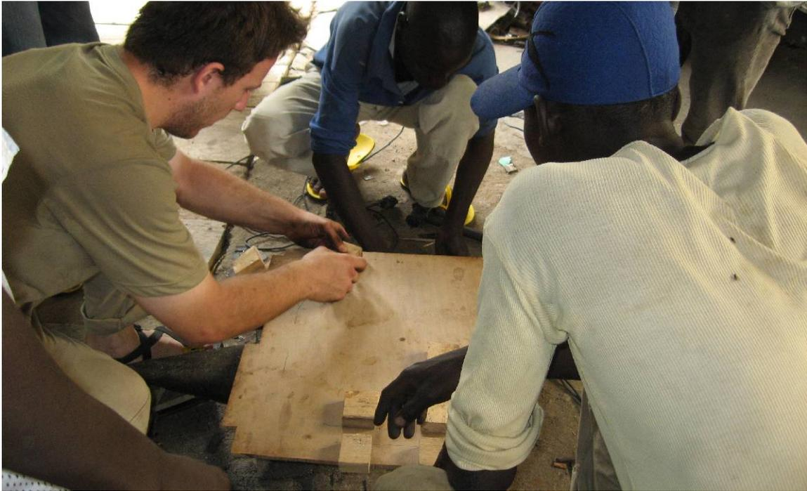
Figure 33: Jigging being constructed from a cheap plank and small scraps of wood.
