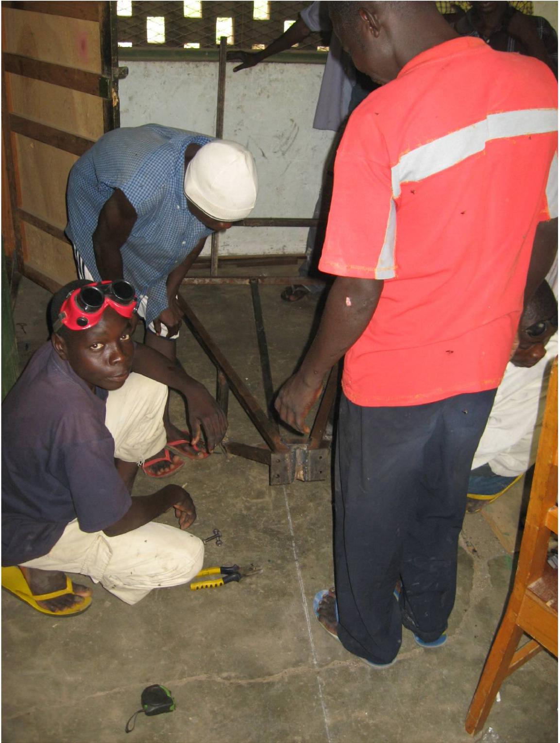
Next, cut the bicycle as shown here to create the front of the vehicle.
