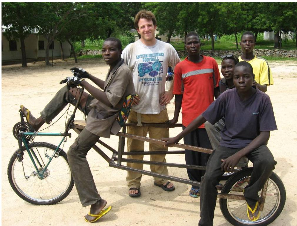
Figure 38: The finished HPUV prototype with the local mechanics and author.
