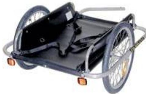
Figure 12: Two-wheeled bicycle trailer produced by Croozer. (BicycleTrailers 2007)
