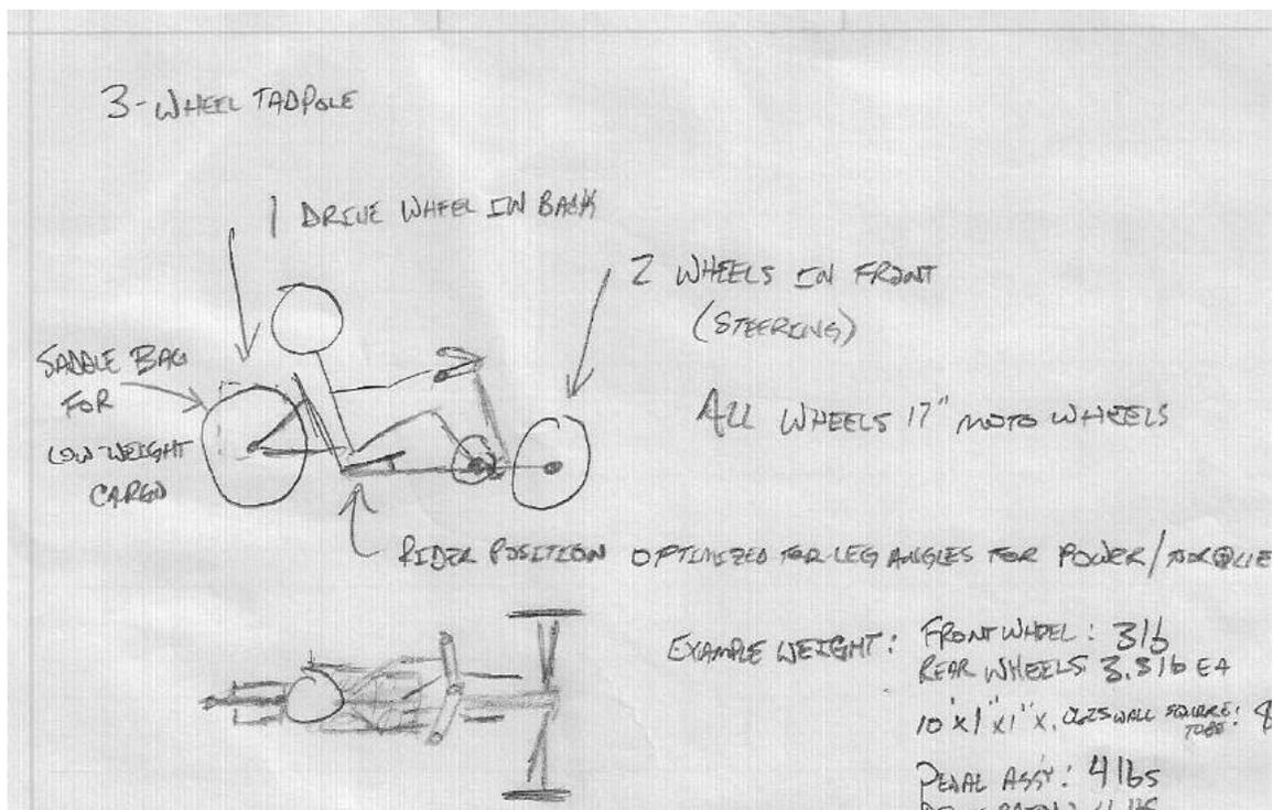
Figure 23: Three-wheeled tadpole-arrangement vehicle concept.
