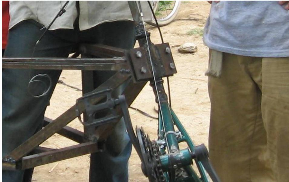
Figure 32: Bolt-on interface on final vehicle, allowing for connection to other implements
