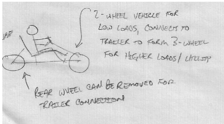
Figure 22: Simple 2-wheeled recumbent concept that attaches to trailer shown in Figure 16.
