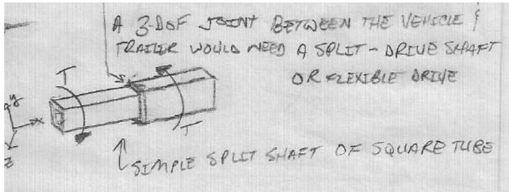
Figure 21: Simple split-shaft design from plain square tube.
