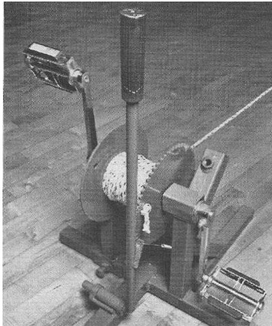
Figure 15: Pedal-powered winch as pictured in *Pedal Power* (McCullagh 1977)
