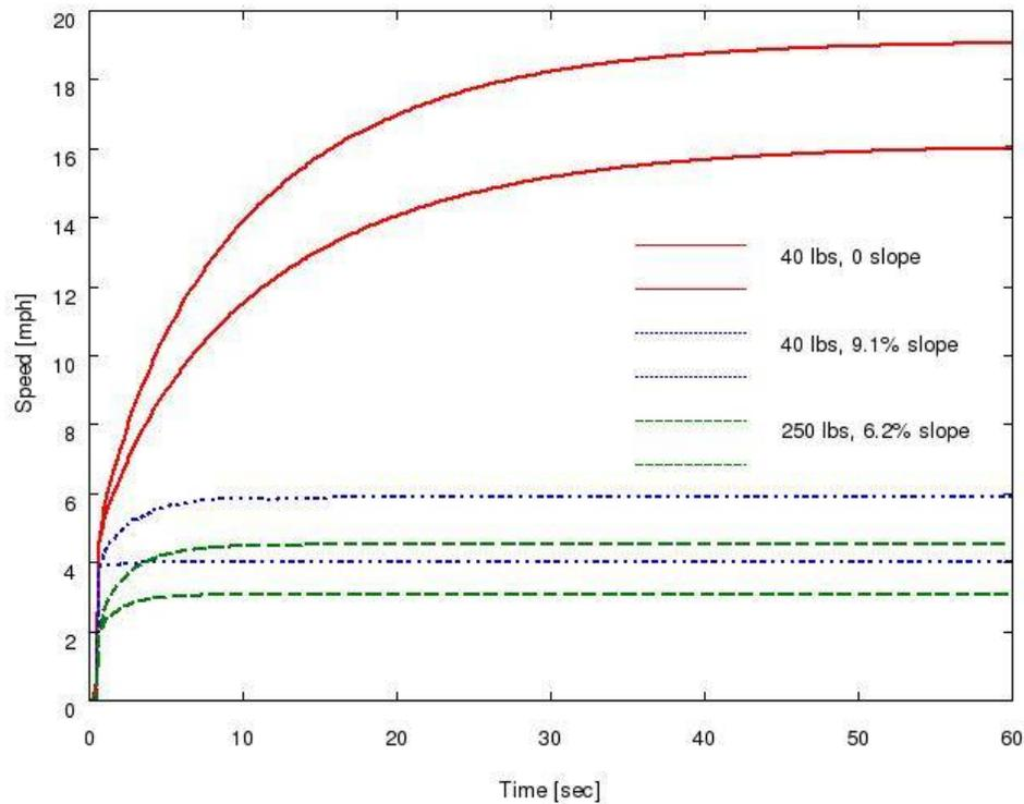
Figure 26: Graph of vehicle performance envelopes for inputs of 0.1 and 0.4 HP at various loading conditions.
