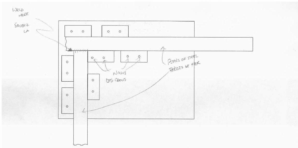
Figure 36: Design drawing of jig structure
