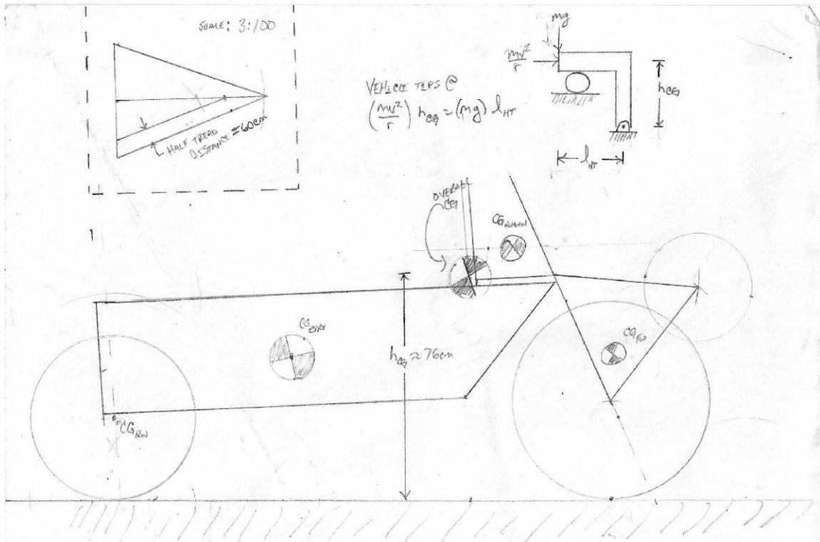
Figure 30: Dimensional sketch showing CG positioning for calculations.
