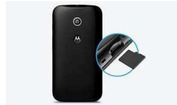
Micro-SD card is inserted into the micro-SD slot.
