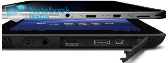
ToshibaThrive AT100 tablet (with USB, mini-USB, HDM ports & jack) against the Toshiba Tablet Galaxy Tab 10" much finer (with microSD, micro-USB, micro-HDM ports & jack). Source: http://www.nextinpact.com/news/65358-toshiba-tablette-tactile-android-fine.htm
