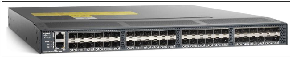
Figure 12-6 Cisco MDS 9148 for IBM System Storage
