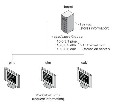
This arrangement, of a server providing centralized services to clients across a network, is known as *client-server computing*.
