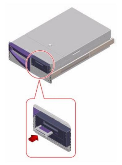
Do not use any cartridge other than a DDS-approved cleaning tape cartridge to clean your tape drive.
