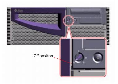
**Note** – Standby current (5 V DC) is still present in the system. To remove all current from the system, remove both AC cables from their back panel receptacles.
