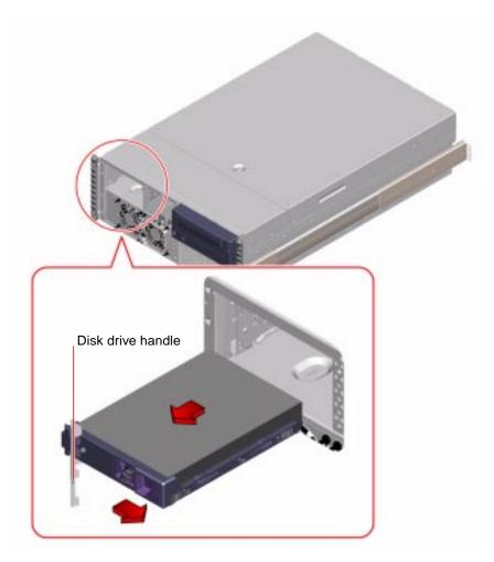
5. Holding the disk drive by the handle, slide it out of the drive bay.
