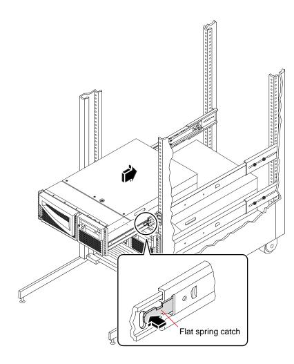
**Tip** – Slide the server in and out slowly and carefully to ensure that the slide assemblies and the innermost glides are working correctly.
