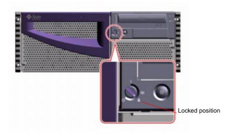
6. Remove the key from the keyswitch, and keep it in a secure place.
