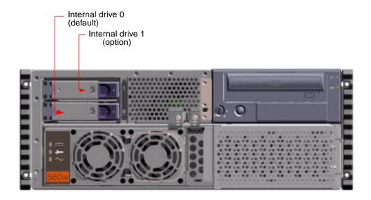
On the right side of each installed disk drive is a green indicator LED. These LEDs indicate the operating status associated with each disk drive. If the drive is being accessed its LED blinks. Continuous LED lighting indicates the drive is ready for the system to use.
