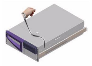
4. Detach both ends of the strap after you have completed the installation or service procedure.
