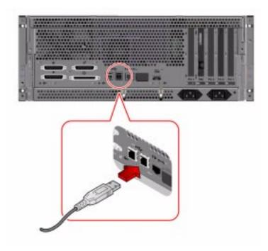
5. Connect the mouse USB cable to any USB port on the back panel.
