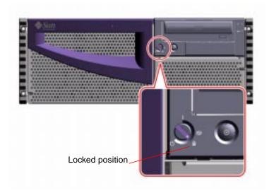
6. Remove the key from the keyswitch, and keep it in a secure place.
