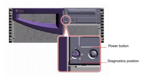
**Note** – The system may take anywhere from 30 seconds to several minutes before video is displayed on the system monitor or the ok prompt appears on an attached terminal. This time depends on the level of power-on self-test (POST) diagnostics being performed.
