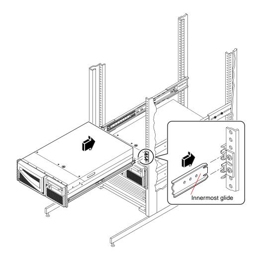
5. On each side of the enclosure, press the flat spring catch mounted on each innermost glide and slide the server all the way into the rack.
