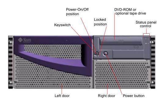
The system's Power button is beside the keyswitch and is controlled by the keyswitch settings. For more information about the keyswitch positions, see "Keyswitch Settings" on page 9.
