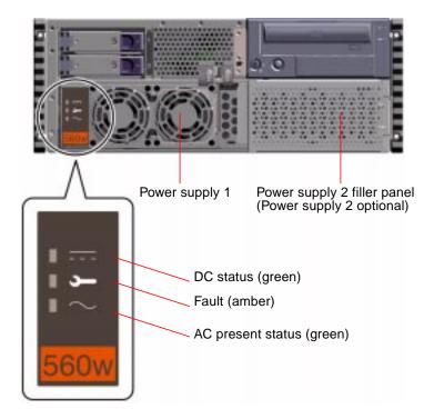
You can use a second supply to provide redundancy, allowing the system to continue operating should one of the power supplies fail. If your server includes a second power supply, connect the second AC power cord to the left inlet (labeled 2
