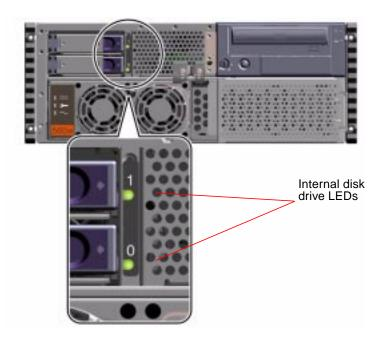
The Solstice DiskSuite software supplied with the Solaris server media kit lets you use *internal* disk drives in two RAID configurations: RAID 0 (striping), RAID 1 (mirroring). You can also configure data drives as hot-spares. For more information on all supported RAID configurations, see "About Disk Array Configurations and Concepts" on page 87.
