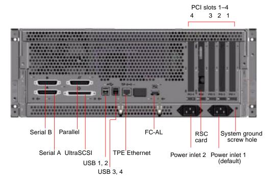
A ground screw hole 0.157 inch in diameter and 0.236 inch deep (4 mm x 6 mm) is located in the lower-right corner of the back panel. Contact your Sun sales representative if you need a grounding strap.
