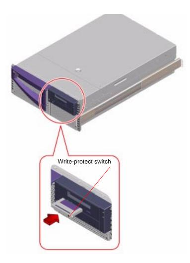
3. Push gently on the cartridge until it is pulled into the drive.
