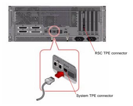
3. Plug in the other end of the cable to the TPE outlet port in the wall or the floor.
