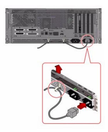
**Note** – If your server includes a second power supply, connect the second AC power cord to the left inlet labeled (2). You may connect the second power supply to the same AC circuit as the first supply. However, for increased system redundancy connect each power supply to a separate circuit.
