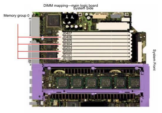
After you have identified the defective DIMM, for more information see the *Sun Fire 280R Server Service Manual*; to replace any defective part(s) contact your qualified service provider.
