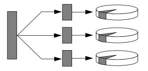
System performance using RAID 0 will be better than using RAID 1 or 5, but the possibility of data loss is greater because there is no way to retrieve or reconstruct data stored on a failed drive.
