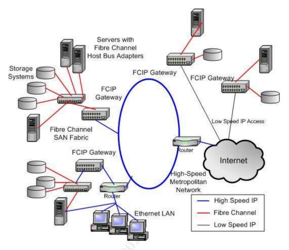
Figure 4: A typical FCIP network configuration.<sup>40</sup>
