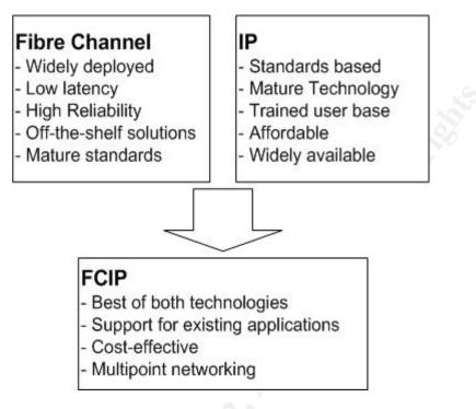
Figure 3: FCIP combines the best benefits of both IP and Fibre Channel technologies. <sup>39</sup>
