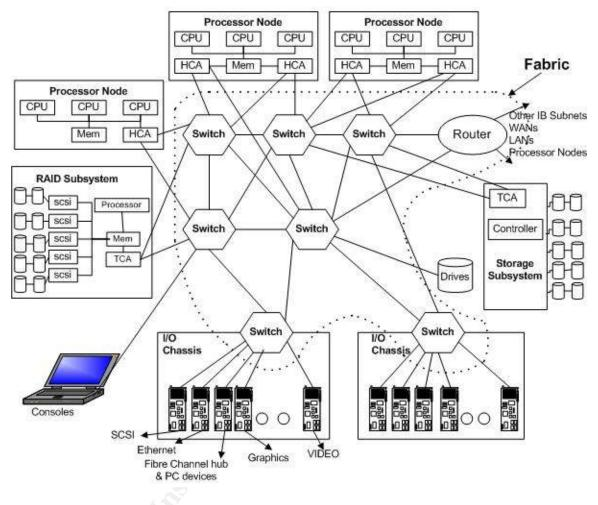
Figure 2: Typical InfiniBand Topologies. <sup>35</sup>
