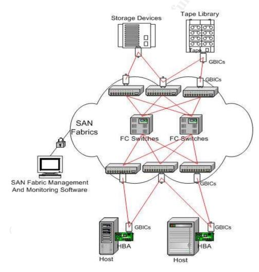
Figure 1: Basic SAN Components.<sup>11</sup>
