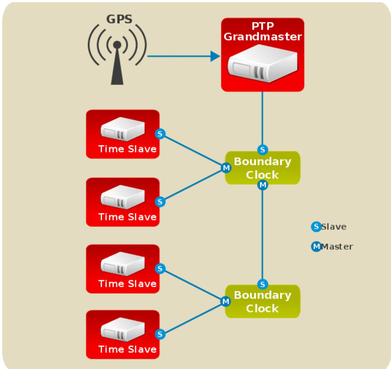
Figure 15.1. PTP grandmaster, boundary, and slave Clocks
