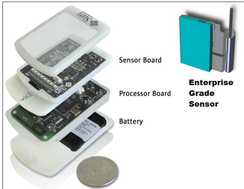
Fairly recently, the SPOT device has evolved into a much more commercially accepted Enterprise grade sensor, which has many applications, such as part of a shipping container tracking solution, where it is a self-contained, self-sufficient unit with a very long, possibly days of, extended battery life which has additional satellite communication and embraces the sensor fusion architecture.
