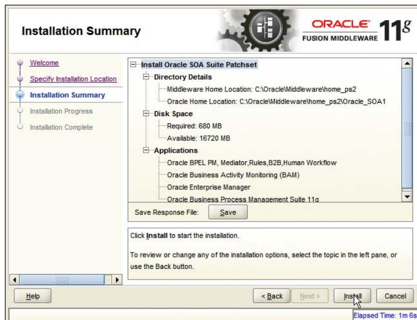
2. Confirm that the installation summary is correct and select **Install**. Wait for the install to complete—it takes a few minutes.
