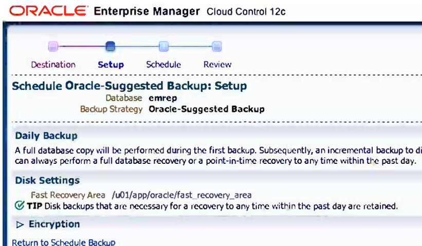
**Figure 13-32.** Choose the Fast Recovery Area as the disk-based backup location
