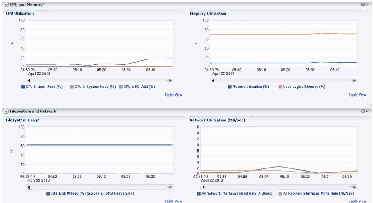
**Figure 9-2.** Host performance information—note the spike in network utilization after 1:44 PM in the bottom-right graph
