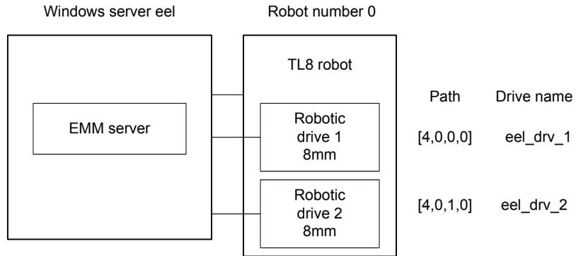
This configuration has a tape library that contains two 8mm tape drives. The robot and drives are connected to a server that runs Microsoft Windows.
