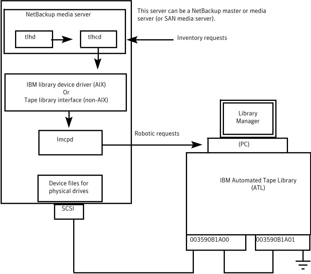
**Figure 9-2** Robotic control and robot connection on separate hosts
