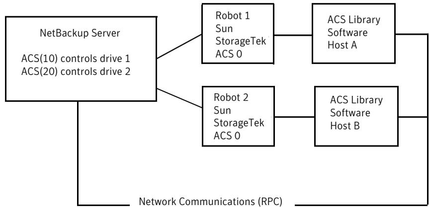
Inventory requests include the volumes that are configured on the ACS library software hosts (Host A for Robot 1 and Host B for Robot 2). The software hosts reside on the robot (ACS 0 for each) that is designated in the Sun StorageTek drive address.
