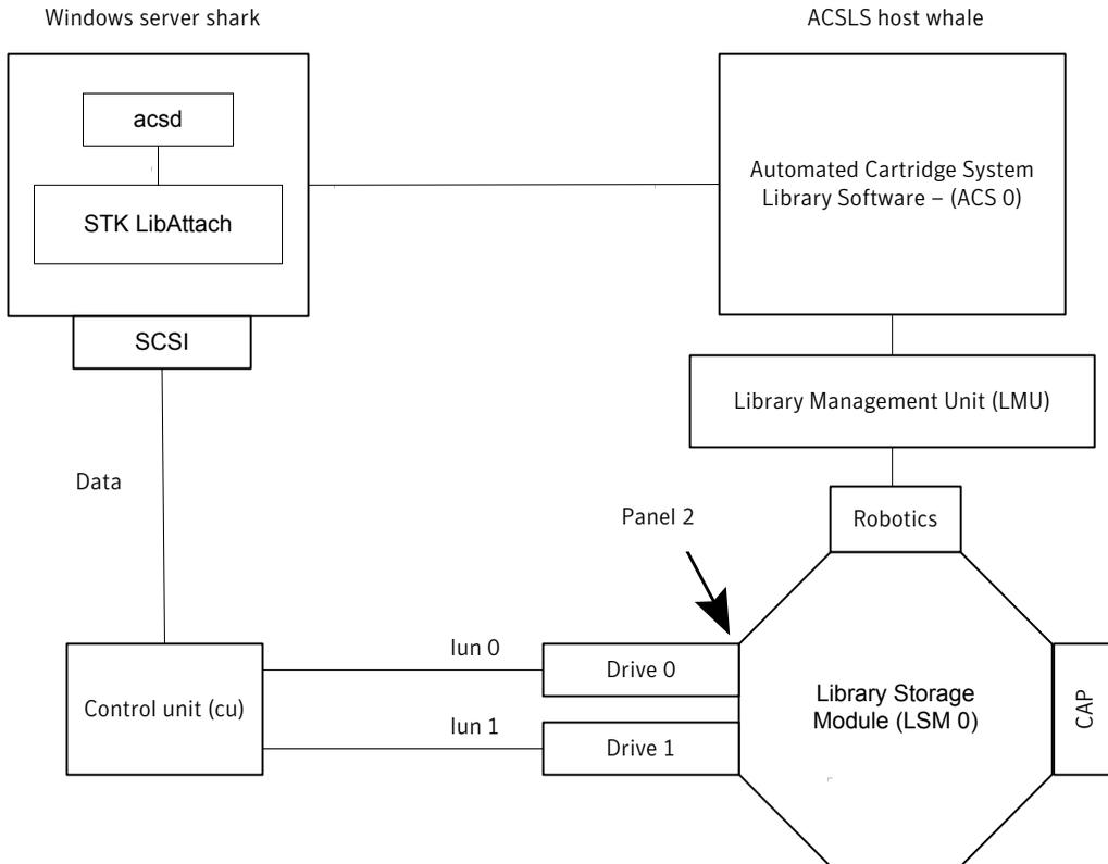
This configuration uses an Automated Cartridge System (ACS) robot for storage. Server shark can be a Windows NetBackup master server or media server.
