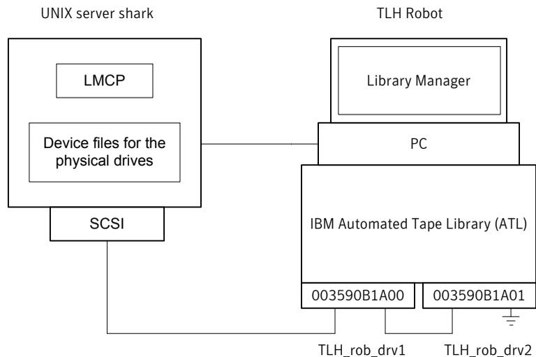
This configuration adds a TLH robot to the configuration. The server shark can be a UNIX (AIX, Solaris SPARC, HP-UX), Linux, or Windows server, and can be a NetBackup master server or media server.
