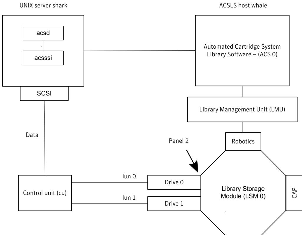
This configuration uses an Automated Cartridge System (ACS) robot for storage. Host shark can be a UNIX NetBackup master server or media server.
