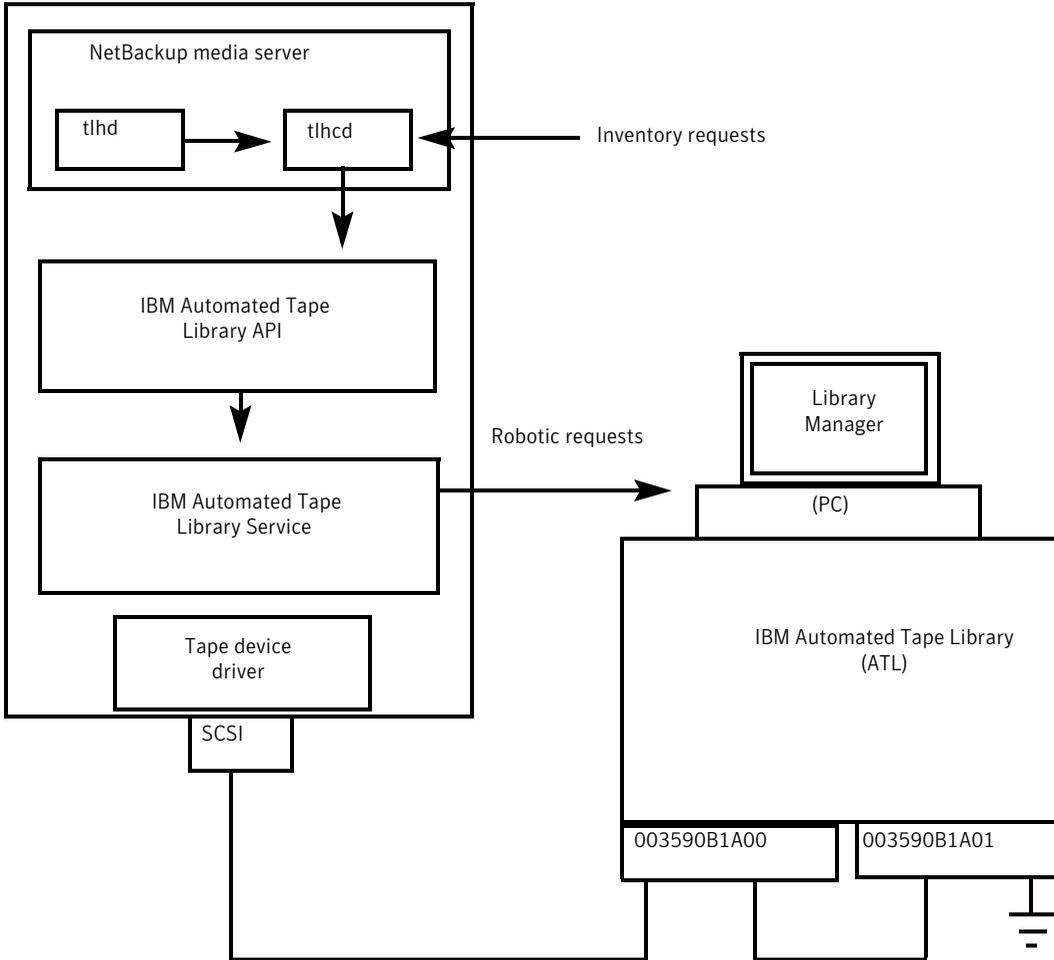
**Figure 9-4** Robotic control and robot connection on separate hosts
