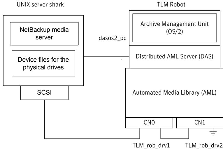
This configuration adds a TLM robot. The device configuration for this robot is similar to the TL8 robot example.
