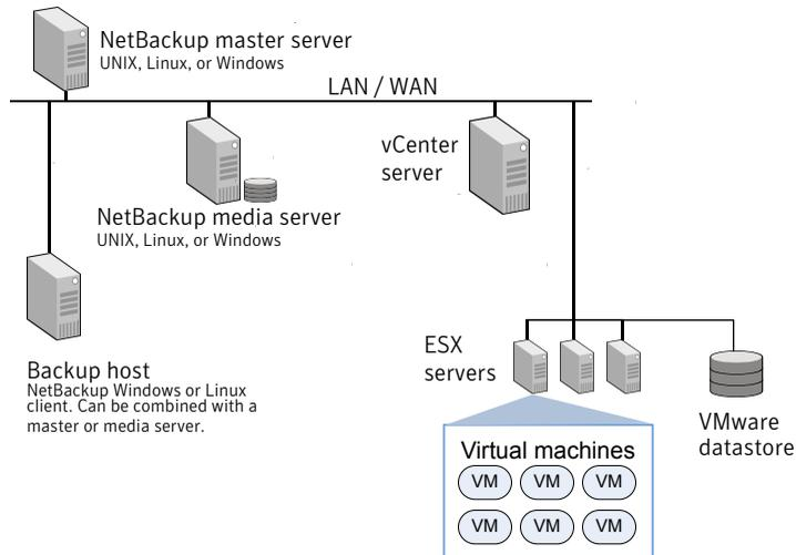
Figure 1-2 shows a NetBackup for VMware environment on a SAN. The backup host accesses the VMware datastore directly over the SAN.
