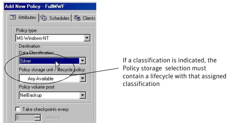
After data is backed up to a storage lifecycle policy with an assigned classification, the data is managed according to the storage lifecycle configuration. The storage lifecycle defines what happens to the data from the initial backup until the last copy of the image expires.
