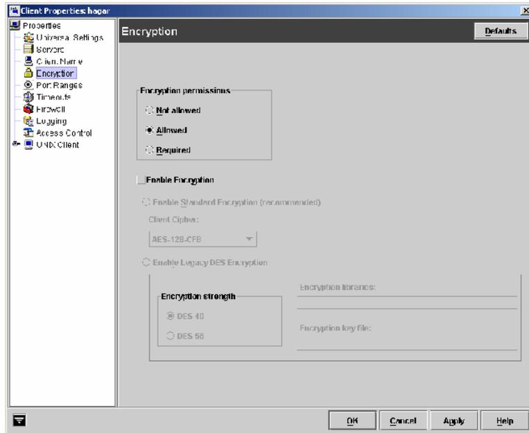
The **Encryption permissions** property indicates the encryption setting on the selected NetBackup client as determined by the master server.
