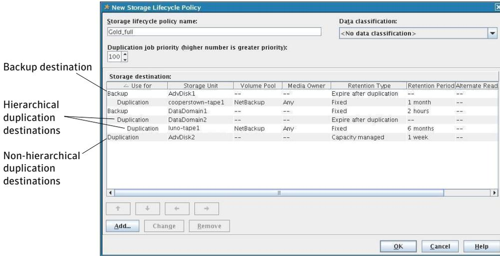
Changing the location of a destination in the hierarchy changes the storage unit that serves as the source for the subsequent copies. Changing the location cannot change the destination type. (For example, make a backup destination into a duplication destination.)
