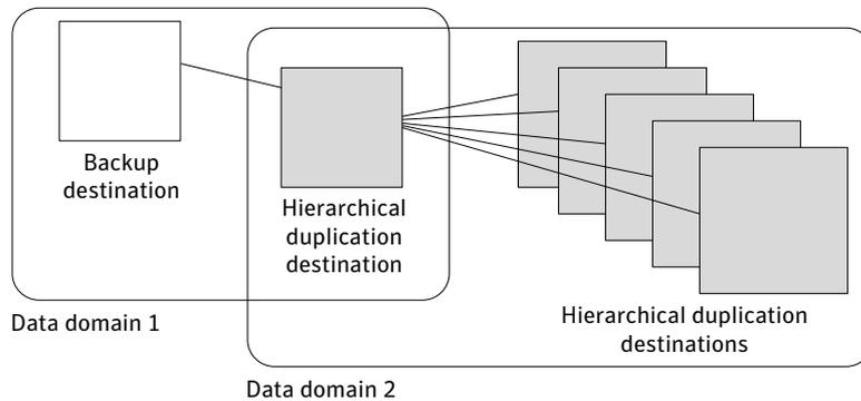
Figure 14-4 shows how the hierarchy of destinations is represented graphically in the **Storage Lifecycle Policy** dialog box. The indentation (or hierarchy) indicates the backup source for each copy. One copy can be the source for many other copies.
