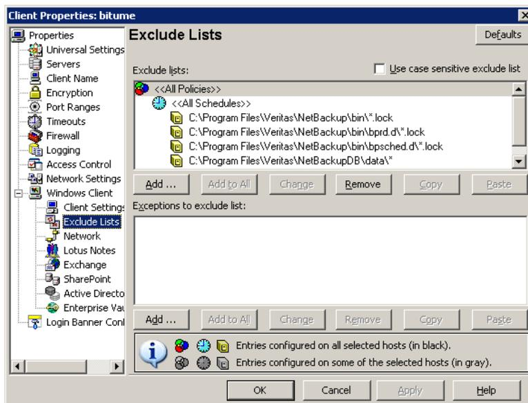
**Exclude Lists** properties apply only to Windows clients. On NetWare target clients, specify the exclude list when the targets are added. NetWare NonTarget clients do not support exclude lists. For more information, see the NetBackup user's guide for the client.
