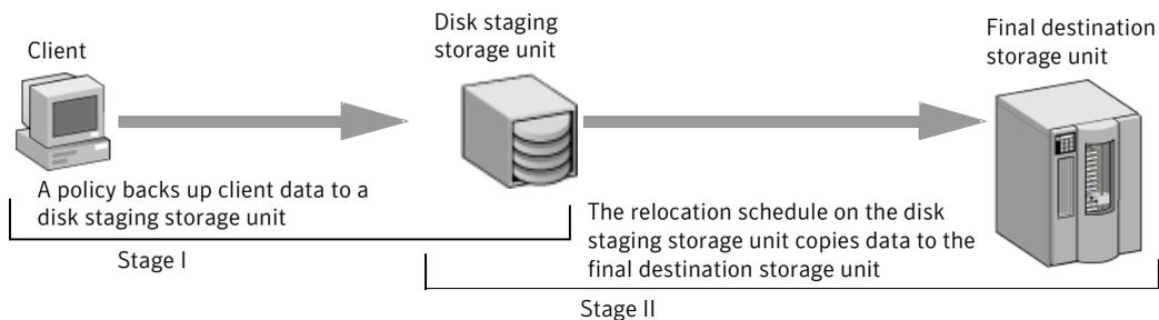
When the relocation schedule runs, NetBackup creates a data management job. The job looks for any data that can be copied from the disk staging storage unit to the final destination. The Job Details in the Activity Monitor identify the job as one associated with basic disk staging. The Job Details list displays Disk Staging in the job's Data Movement field.
