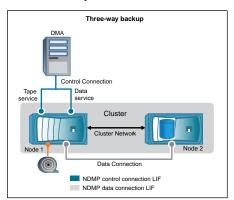
Using the affinity information about volumes and tape devices, the DMA (backup application) performs a local NDMP backup on the volume and tape device located on Node 1 in the cluster. If the volume moves from Node 1 to Node 2, affinity information about the volume and tape device changes. Hence, for a subsequent backup the DMA performs a three-way NDMP backup operation. This ensures continuity of the backup policy for the volume irrespective of the node to which the volume is moved to.
