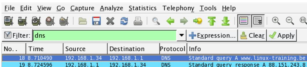
The details in wireshark will say the DNS query was inside a udp packet.
