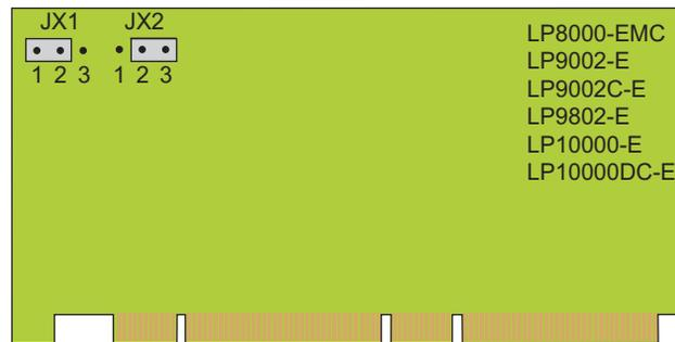
2. With host system power removed, install the HBA as instructed in the server documentation. The card installs into a single PCI bus slot.
