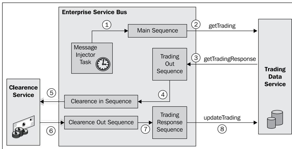
Synapse supports tasks that can be run periodically. A task can be written in Java and configured in the `synapse.xml` file.
