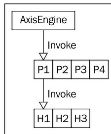
A phase is designed to support phase rules. Phase rules tell Axis2 where to put handles in the execution chain. As we will see later, there are rules like `phaseFirst` and `phaseLast`. So in a `Phase`, there are reserved slots to hold both the phase first and phase last handlers. The rest of the handlers will be kept in a different list. A phase can be graphically represented as follows:
