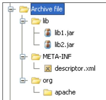
As mentioned earlier, in the case of a service the `descriptor.xml` file would be `services.xml`. So in the service archive file, you can find a file called `services.xml` inside the `META-INF` directory. On the other hand, for the module archive, `META-INF` will have a file called `module.xml`.
