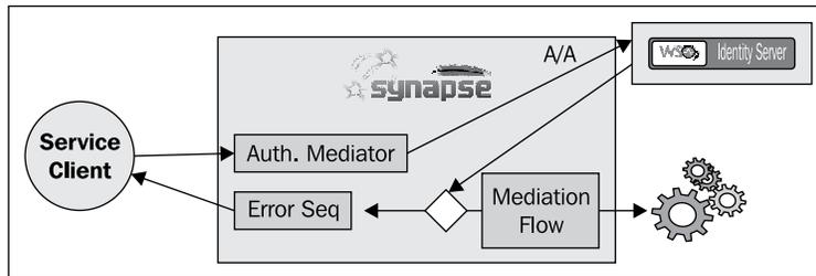
The second pattern is where the service client itself can talk to the identity management server, as shown in the figure below. Here, WS-Trust or some other security token-based protocol is used. The flow sequence is as follows:
