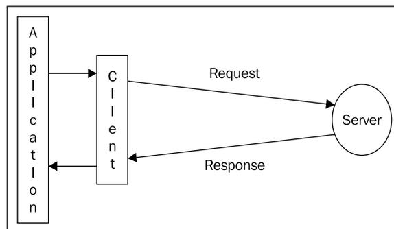
In the case of asynchronous type invocation, the user application (for example, GUI) does not block, so the user can continue working. Axis2's way of utilizing a service in asynchronous is shown in the following figure:
