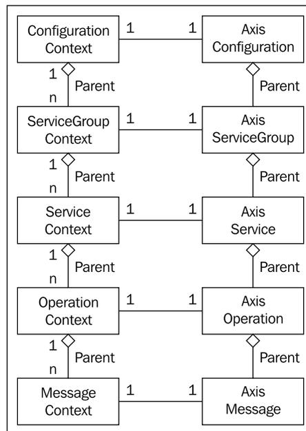
As you can see on the left-hand side, the top most component of the hierarchy is `ConfigurationContext`. The only difference, when `ConfigurationContext` is compared to other contexts, is that it is the only context that exists in the system before receiving a message. `ConfigurationContext` has a reference to an `AxisConfiguration`, and to create `ConfigurationContext`, it is required to have an `AxisConfiguration` available.
