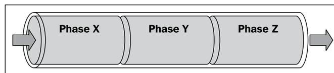
If the message has gone through the execution chain without having any problem, the engine will hand over the message to the message receiver in order to do the business logic invocation. After this, it is up to the message receiver to invoke the service and send the response if necessary. The following figure shows how the message receiver fits into the execution chain:
