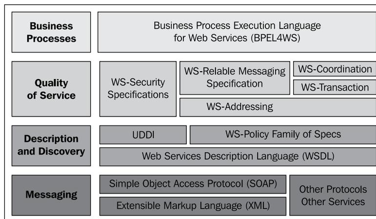
The messaging standards are intended to give the framework for exchanging information in a distributed environment. These standards have to be reliable so that the message will be sent only once and only the intended receiver will receive it. This is one of the primary areas where research is being conducted, as everything depends on the messaging ability.
