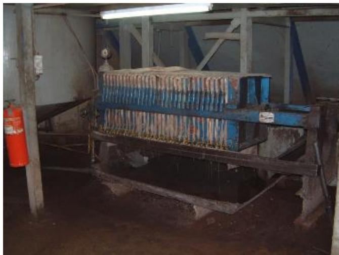
Figure 8: Typical filter press. Photo: Tony Swetman
