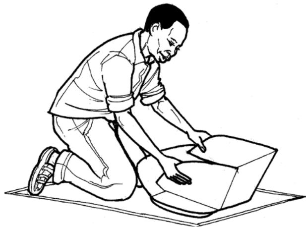
Assemble the cooker in a shaded area, to avoid dazzling your eyes. Lay the panel flat with shiny side up, and the wide back panel away from you. Tilt the back panel towards you and carefully slide the ends of its flaps into the slots on the shorter front panel that is nearest to you. As you do this, you will also need to tilt the front panel up. Clamp the inserted flaps, on the underside of the front panel, using clothespins or similar device. You are ready to cook!
