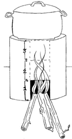
**LESSON 2. BURN WISE** A fire that burns only the tips of wood will burn hotter and make less smoke. It will also use much less fuel. The temperature of the fire depends on how many tips of wood are burning. Well-designed stoves help users meter the amount of fuel they use, feeding in only as much as they need to cook their food.
