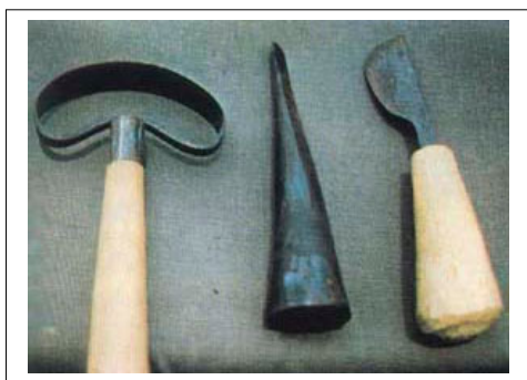
Photo 5.4 Indonesian tools used in benzoin tapping.
