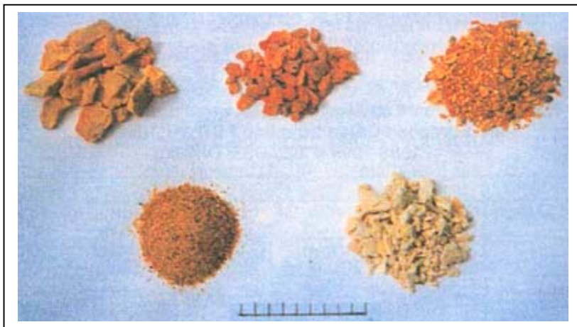
Photo 7.1 Siam benzoin (Lao PDR) Scale: 1 cm divisions Top (L→R) Grade A, B and C Bottom (L→R) Grade D and fresh mixed
