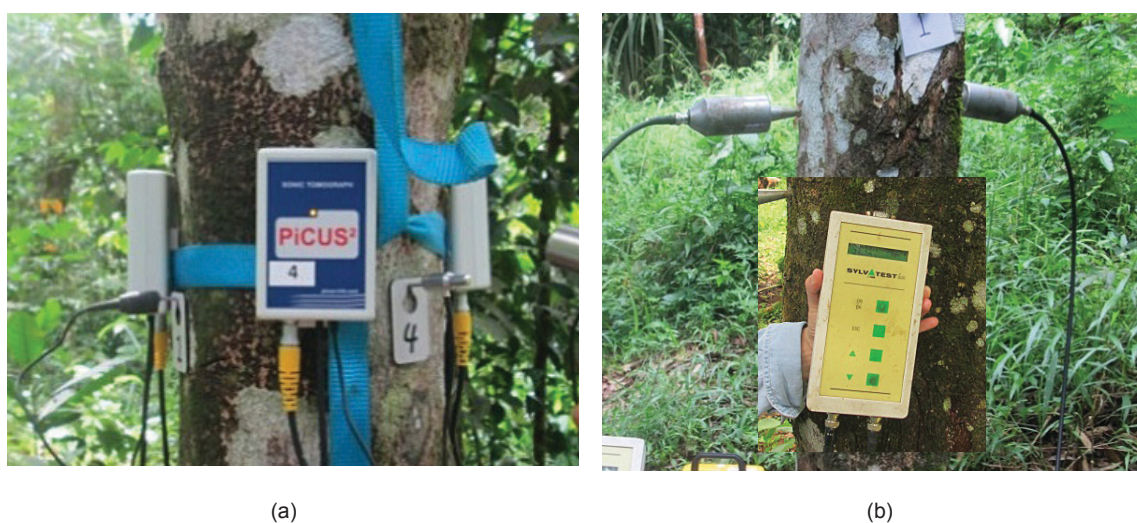
Figure 2 (a) Sonic or stress wave and (b) ultrasonic wave testing methods applied on an Aquilaria tree
