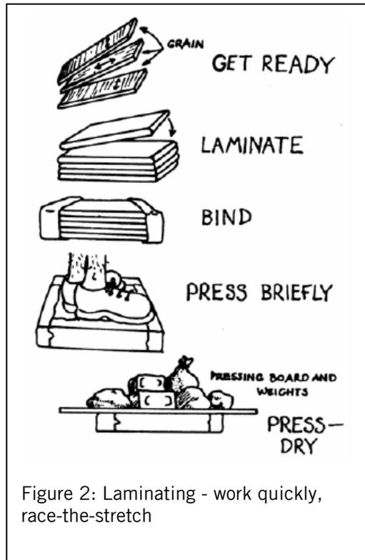
Figure 2: Laminating - work quickly, race-the-stretch
