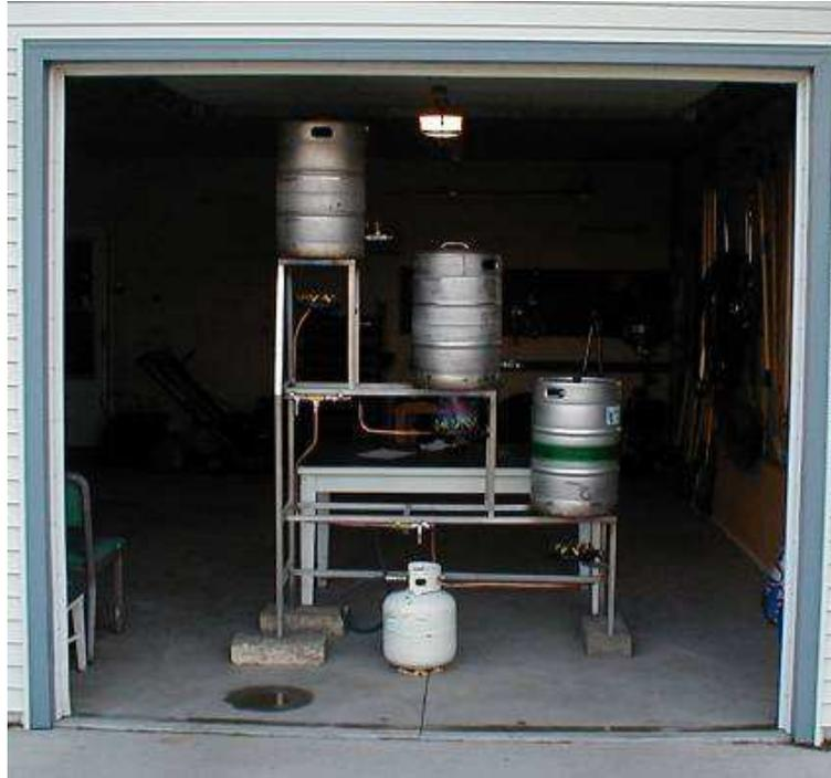
Fig 11. – Three tier gravity feed set-up
