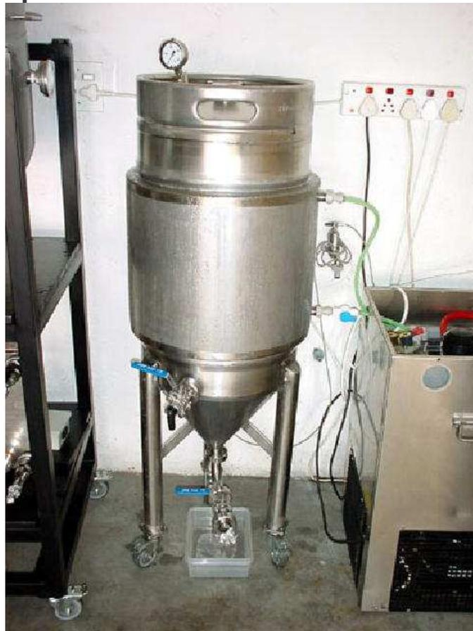
Fig 10. – Conical fermenter
