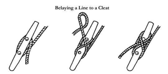
Cleats have been used for centuries by seamen to secure boats to a dock, as well as securing halyards and other running rigging on the boat.
