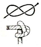
A figure eight knot is very quick and easy to tie. It is used like the overhand knot, as a stopper knot in the end of a line, or sheet, to prevent ropes from escaping. It can also be used to attach rope halyards, to the sails. It never jams, however much pressure is applied, and can be untied easily, even if wet.
