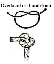
Overhand or thumb knot, is the simplest knot. It is used to stop the end of a rope from running through a block or up the mast.
