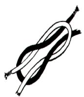
The square knot is the best known sailors' knot. It is really just two overhand knots. It is useful for joining small ropes together, tying sail covers, reefing, lashing, and for tying in battens.
