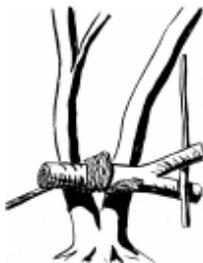
A bush windlass, capable of taking a very heavy strain on a rope can be made by selecting a site where a tree forks low to the ground, with the fork facing the direction in which the pull is required. Alternatively, a stout fork can be driven in and anchored with the "1-2-3" method.
