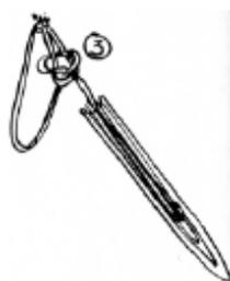
At one end of the string tie a loop and place the knot on a conveniently high nail or hook. The mesh stick is put under the loop and the needle with cord passed through as in Fig. 3. The needle and cord are passed in front of the loop formed in Fig. 3 and under the original loop, while at the same time the other end of the cord is held on to the mesh stick with the thumb of the left hand. The knot is pulled taut.
