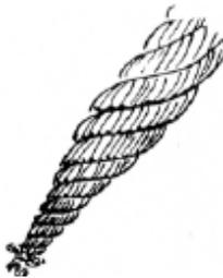
The rope is unlaidd and a tie put on to prevent it unlaying further. The strands are thinned down gradually, and relaid again. The end may be stiffened with a small stick or piece of wire. The end can be finished off with any of the [crown](#) or [wall](#) knots.
