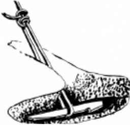
The only way to anchor a rope into soft sand is to attach it to a peg, and bury the peg in the sand.
