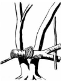
A bush windlass, capable of taking a very heavy strain on a rope can be made by selecting a site where a tree forks low to the ground, with the fork facing the direction in which the pull is required. Alternatively, a stout fork can be driven in and anchored with the "1-2-3" method.
