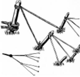
A secure anchor in open ground can be obtained by driving a stout stake well into the ground. The rope is later fastened to the base of this stake.
