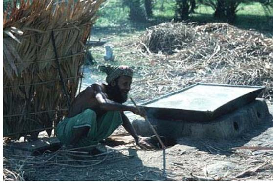
Figure 3: A simple open pan used for processing the juice extracted from the sugar.
