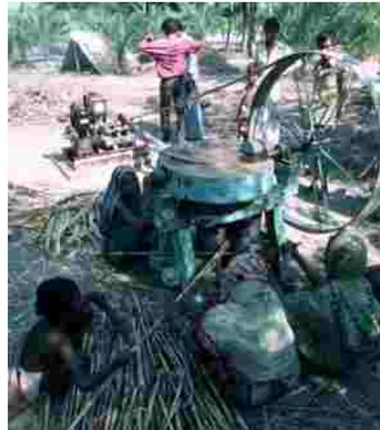
Figure 2: A Diesel powered cane crusher with three vertical rollers in Bangladesh. Photo: Neil Cooper
