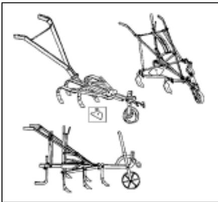
Fig. 7-38: Expandable cultivators. Top left: "Houe Manga" manufactured by UPRAMA, Togo. Top right: "Rhino" cultivator manufactured by Northland Engineering, Zambia. Lower left: Interrow cultivator developed by CAMERTEC, Tanzania. Sources: after ILO, 1983g and UPRAMA, 1986
