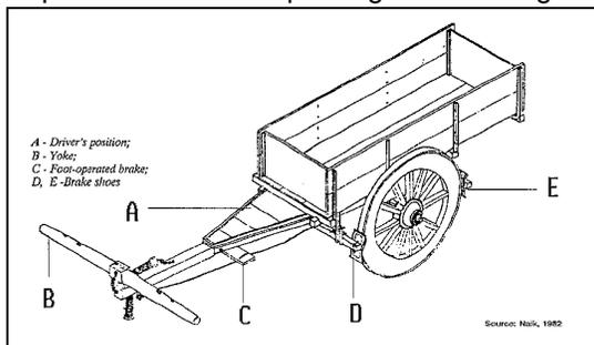
Fig. 8-23: Modified Indian cart design with braking system.
