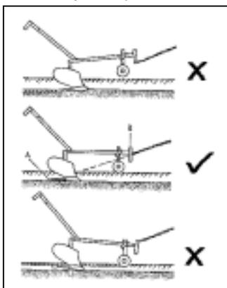
Fig 2-5: Pitch adjustment of a plow (exaggerated).
