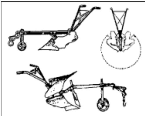
Fig 7-19: Reversible plows. Top: Inexpensive reversible design that is a,uite widely used in India, showing the method of rotating the mouldboard to the other side at the end of a row. Bottom: A more expensive design of plow with two bodies that are alternately swung into place. Designs such as this have been tested in several African countries, but have generally been forma too heavy and expensive for use in the local farming systems. Source: after: Hpfen, 1969;CEEMAT, 1971
