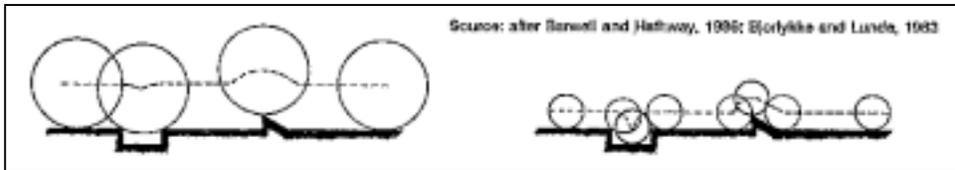
Fig. 8-12: Diagram illustrating how large-diameter wheels (left) are better able to negotiate ruts and holes than small-diameter wheels (right). The ability of a wheel to accept poor conditions is dependent not only on wheel diameter, but also on the width and type of tread and the strength, weight and elasticity of the tyres or wheel rims.
