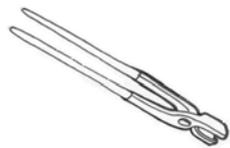
**Tongs** – Used to hold material when it has been heated and is ready for work. These can be made in the forge, for different pieces of work. The heads can be shaped to grip different sizes and shapes of material.
