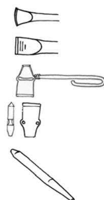
**Hot Chisel** – Used for cutting hot metal, by striking with a hammer. This tool is not hardened and should not be used to cut cold material, only heated.
