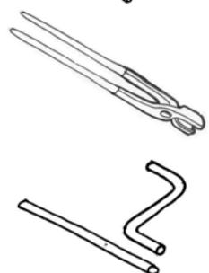
**Tongs** – Used to hold material when it has been heated and is ready for work. These can be made in the forge, for different pieces of work. The heads can be shaped to grip different sizes and shapes of material.
