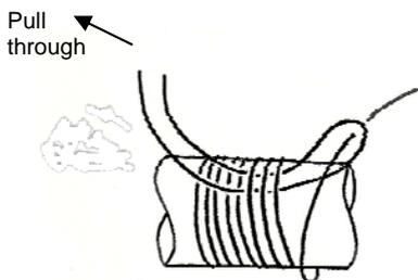
Figure B3b: Finish of binding
