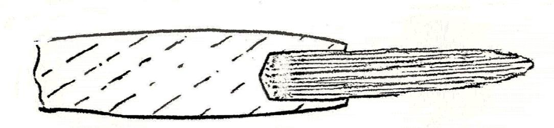
Figure C4: Preformed knot fitted to handle
