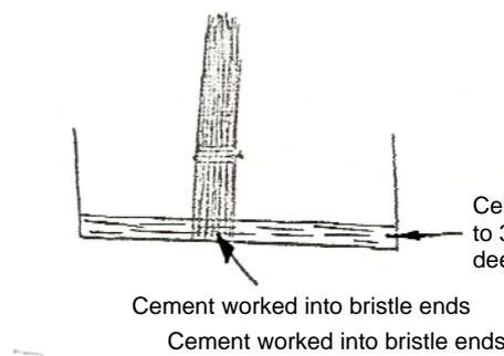
Figure A3: Cementing the "knot"
