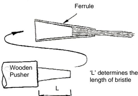
Figure A4: Fitting the "knot" to the ferrule
