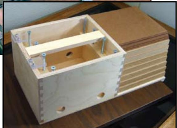
Assembled Sharpening System box
