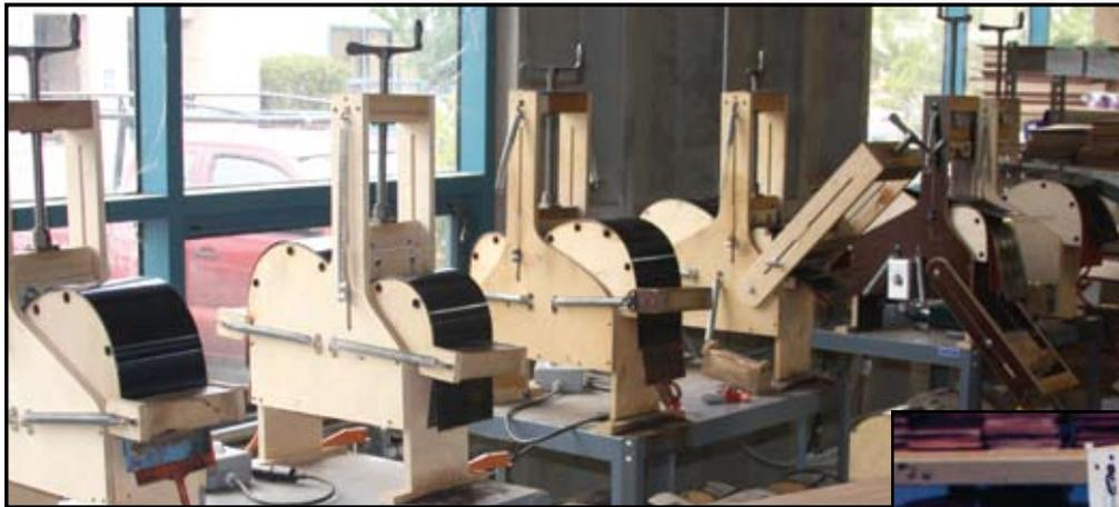
**LEFT:** Universal Side Bending Machines used for bending services in our LMI workshop.
