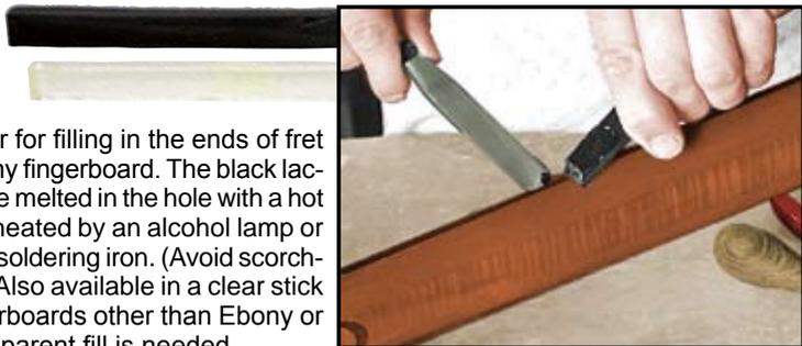
A time-saver for filling in the ends of fret slots in an Ebony fingerboard. The black lacquer wax can be melted in the hole with a hot chisel or knife heated by an alcohol lamp or a conventional soldering iron. (Avoid scorching the wood.) Also available in a clear stick for use in fingerboards other than Ebony or wherever transparent fill is needed.
