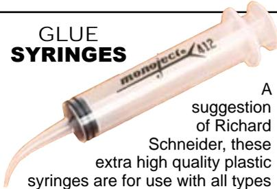
A suggestion of Richard Schneider, these extra high quality plastic syringes are for use with all types of adhesives. The tapered spout is curved for easy access to difficult-to-reach gluing surfaces. The tip tapers to a .030" hole and can be cut along its length to suit the job. The syringes are reusable after careful cleaning. Approx. 3" long; 5/8" diameter; Glue capacity: approx. 1 oz.
