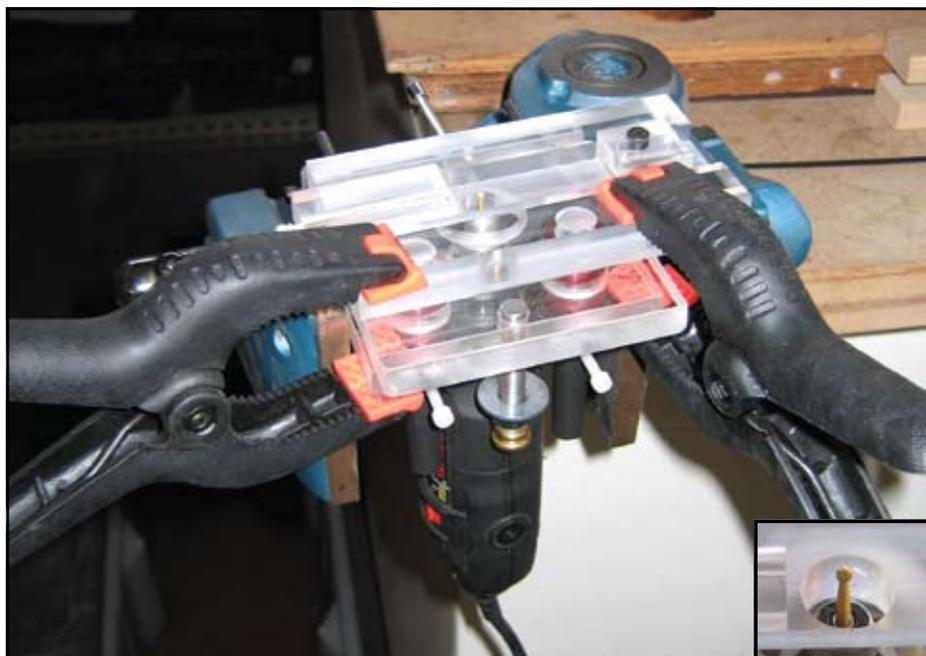
Right: Bridge Pin Groover on the underside of a Dremel® router base.
