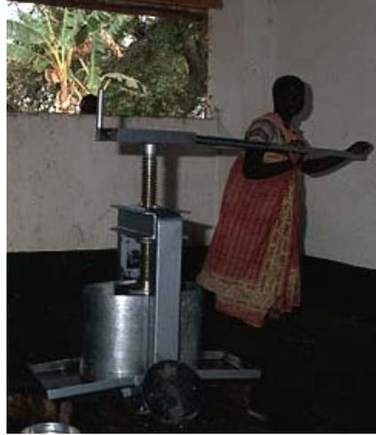
Figure 4: A manual screw press
