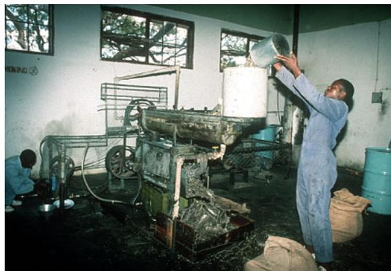
Figure 5: Tinytech oil expeller in operation in Zimbabwe.
