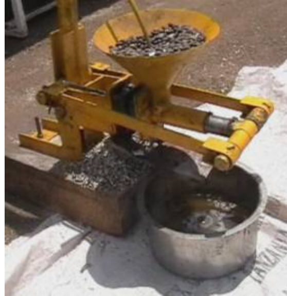
Figure 4-4 Close-up of the Bielenberg pressing mechanism. Notice the automatic discharge of the pressing chamber and the stopper in the seed funnel [12]
