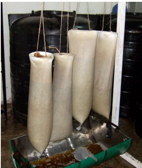
Figure 4-11 Left top: SVO filtration of cooking oil on the site of German supplier Monopoel. Right top: simple filtration setup using bag filters (photo: Diligent Tanzania Ltd.). Left bottom: improved setup for bag filters (photo: Diligent Tanzania Ltd.). Right bottom: employee collecting an oil sample for analysis after filtration (photo: Diligent Tanzania Ltd.)
