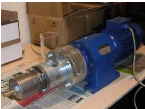
Figure 4-7 The Danish BT press is an example of a cylinder-hole type press. Notice the nozzle, left in front [10]
