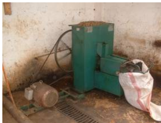
Figure 4-8 The Sundhara oil expeller is a representative of the strainer type press. On the right the choke adjustment [12]
