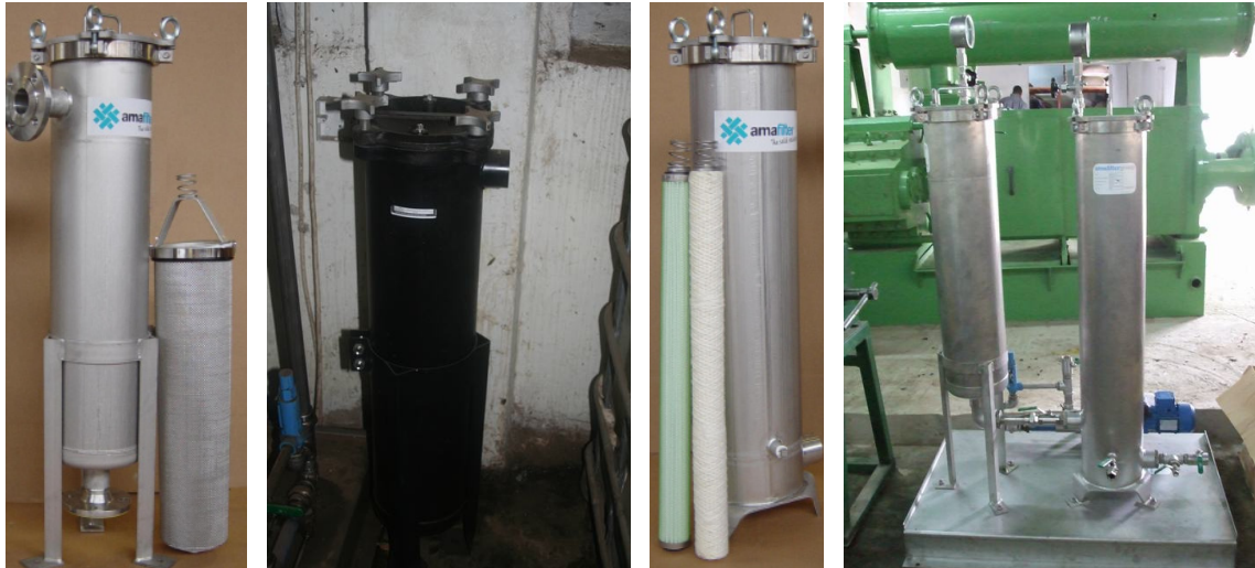
Figure 4-15 Bag- and candle filters. From left to right: 1) Filter housing with filter basket. The filter bag is inserted in the basket and need cleaning every 14 days. 2) Bag filter housing unit for a bag filter (without pump or storage), at Diligent Tanzania Ltd. 3) Candle filter housing with filter candles. The candles need to be replaced by new ones every 6-8 weeks. 4) Combined setup of a bag and candle filter (photos: 1&3 www.amafilter.nl , 2&4 Diligent Tanzania Ltd.)
