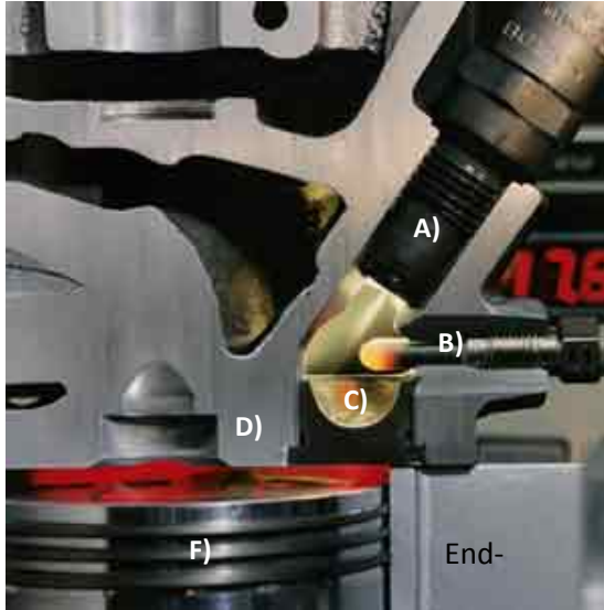
Figure 5-6 Cross section of an IDI combustion chamber. A) single-hole Injector, B) glow plug, C) pre chamber, D) cylinder head, E) piston, F) cylinder wall (photo: Robert Bosch GmbH)
