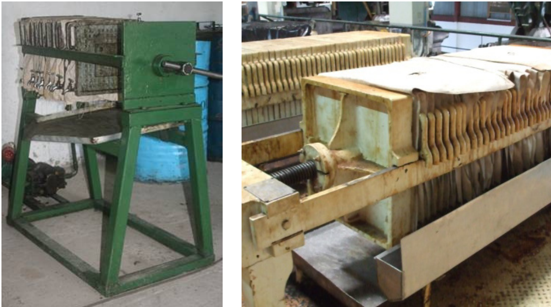
Figure 4-13 Plate filters. Left: Small system (150 l/h) produced by TEMDO Tanzania, installed at Diligent Tanzania Ltd. Right: plate filter for food industry, capacity around 1000 l/h.
