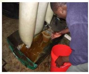
**Figure 11** – Left top: SVO filtration of cooking oil on the site of German supplier Monopoel. Right top: simple filtration setup using bag filters [picture Diligent Tanzania Itd.]. Left bottom: improved setup for bag filters [picture Diligent Tanzania Itd.]. Right bottom: employee collecting an oil sample for analysis after filtration [picture Diligent Tanzania Itd.]
