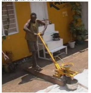
Figure 2 – the Bielenberg ram press operated at Figure 3 – close-up of the Bielenberg pressing Kakute Ltd., Tanzania [12]
