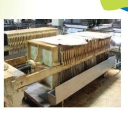
Figure 14 Plate filter with capacity of 150 Figure 15 Plate filter for food industry, capacity liters/hour. At Diligent Tanzania ltd. Produced by **TEMDO** Tanzania.
