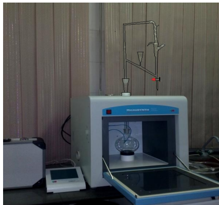
Fig. 2. Adapted microwave distillation apparatus
