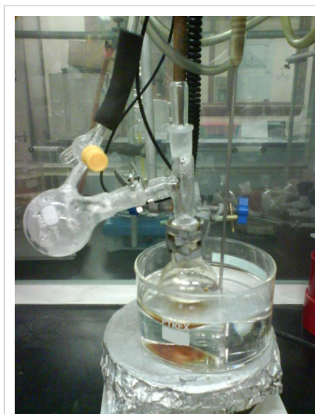
Dimethyl sulfoxide usually boils at 189 °C. Under a vacuum, it distills off into the receiver at only 70 °C.
