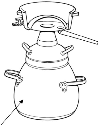
This small still has a combined condenser on the top of it, shown in section. Cold water is put into the open pan and condensation collects in the dome.
