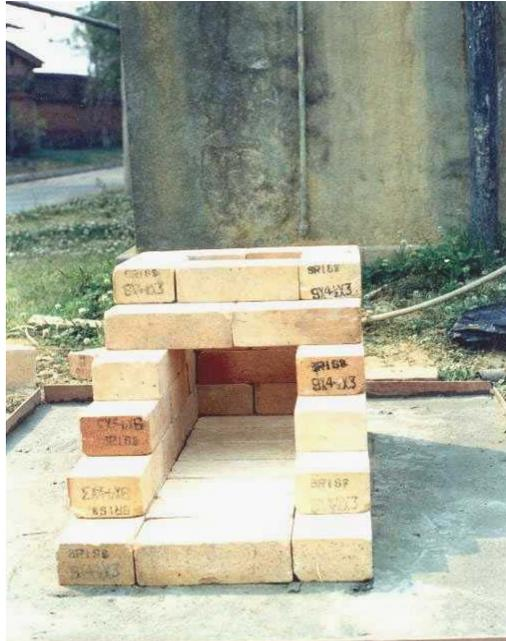
Figure 3: Channel opening between combustion chamber and flue outlet.
