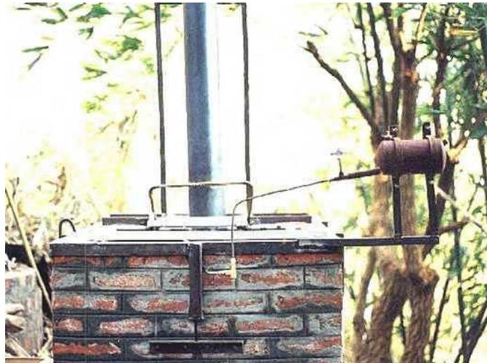
Figure 12: Two litre fuel tank fitted to top framework
