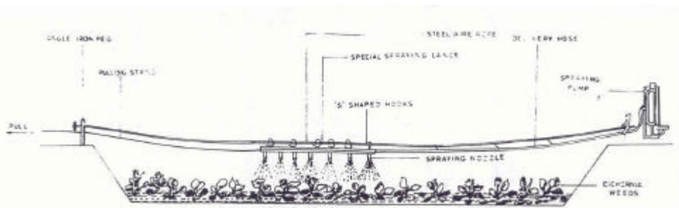
Fig.25. Special spraying arrangement for sites unmanageable from the banks
