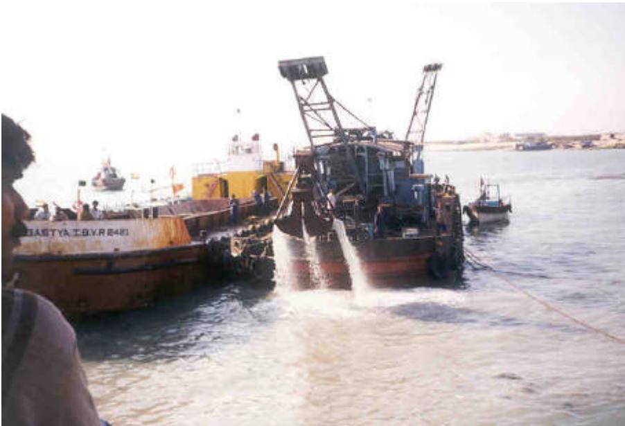
Fig.7. Dredging essentially meant for desilting along shores also helps in removal of aquatic weed vegetation
