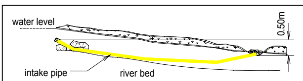
Figure 10-1 The simplest intake design is a pipe anchored in the flow
