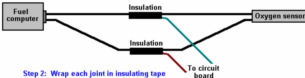
**Step 2: Wrap each joint in insulating tape**
