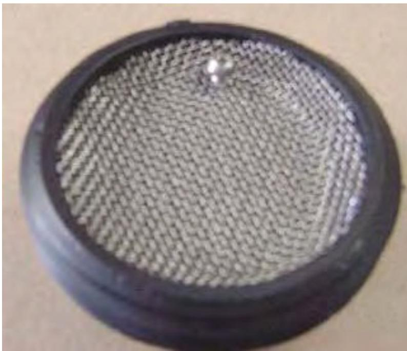
After fitting the mesh tightly into the cap, mount it with a 10/32 stainless steel screw on the opposite side to the 1/4" tapped hole for the barbed fitting. This is a flame arrestor, so make CERTAIN that the entire inside is covered tightly. Note that the sides wrap up. Turn each layer to cross the grain of the mesh.
