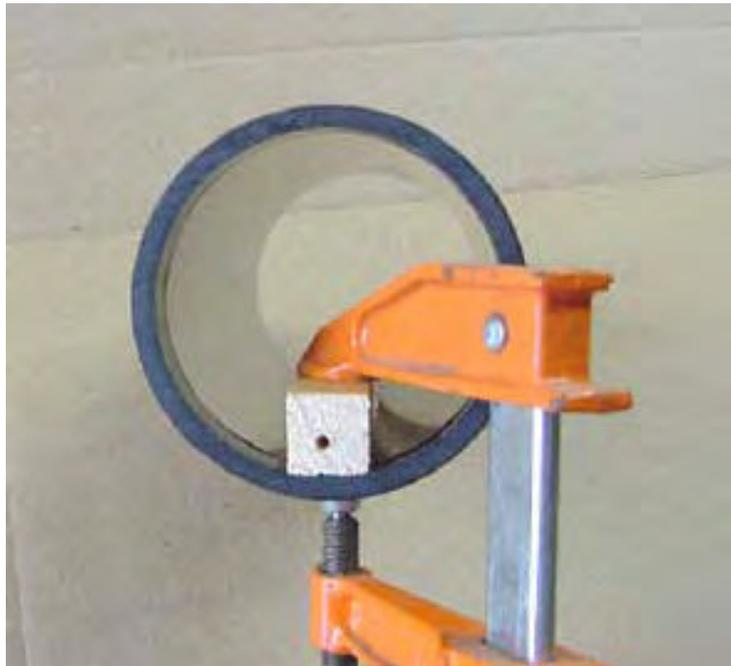
Clamp securely and drill two 0.165" holes, one on either side, perpendicular to each other, as best you can.
