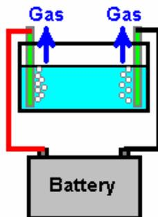
Here, a current flows through the liquid inside the electrolysis cell, moving from one plate to the other. The current breaks the bonding of the water molecules, converting the  $H_2O$  into hydrogen H and oxygen O. There are various forms of hydrogen and oxygen and mixtures of the two. H atoms on their own are called "monatomic"
