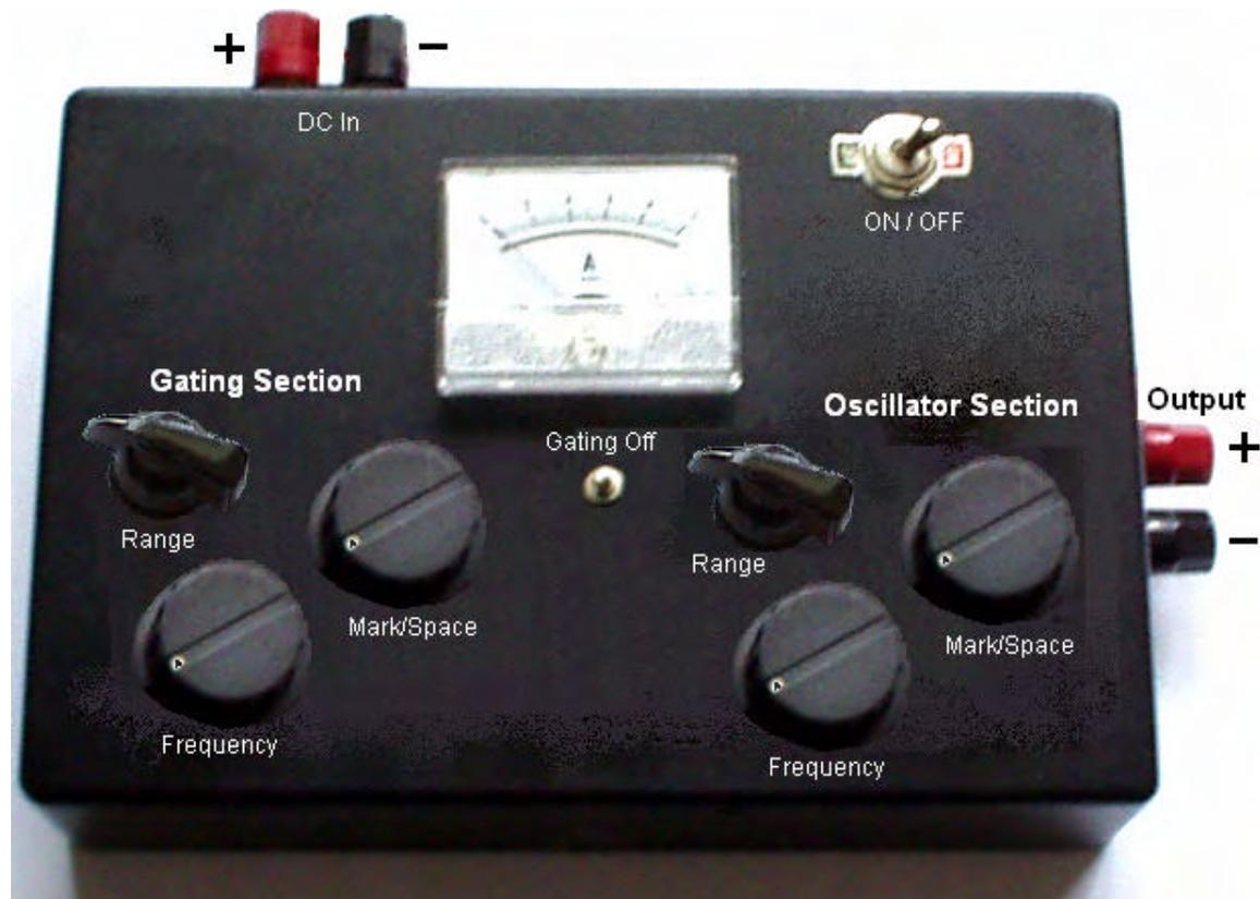
The ammeter shown here is not really necessary and can be omitted.
