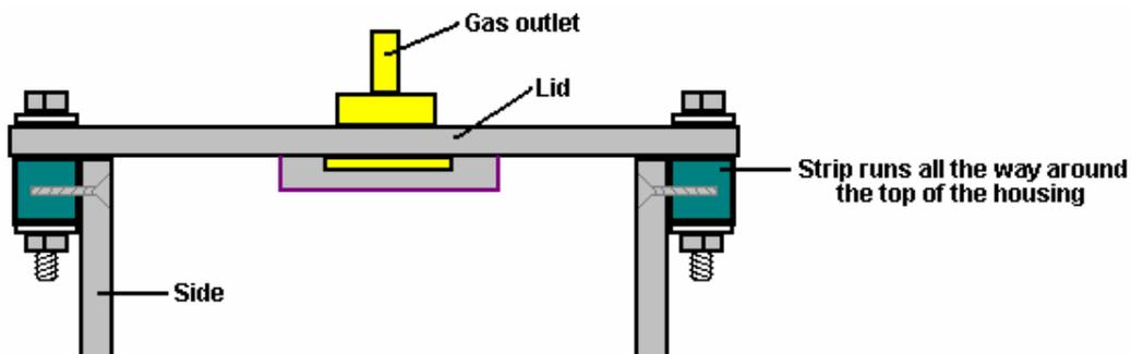
A gasket placed between the sides and the lid would assist in making a good seal when the lid is bolted down. The gas outlet pipe is located in the centre of the lid which is a position which is not affected if the unit is tilted when the vehicle is on a steep hill.
