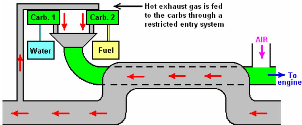
The use of carburetors is important since using a bubbler as suggested in the free plans on the internet, creates problems as the lighter fractions of the fuel get taken first which is exactly what we don't want to happen. The carburetors have the massive advantage that they feed all fractions of the fuel together and so the remaining fuel is always in the correct proportions.
