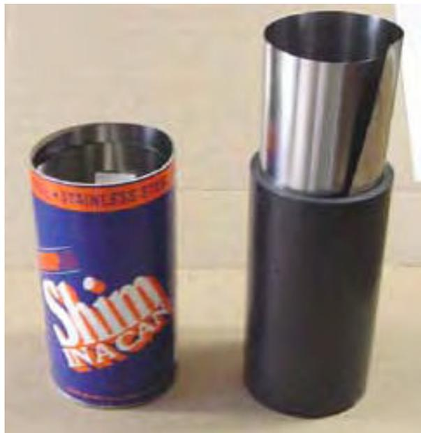
Cut and fit shimstock into ABS tubing, 11" works well as this gives a 1" overlap.
