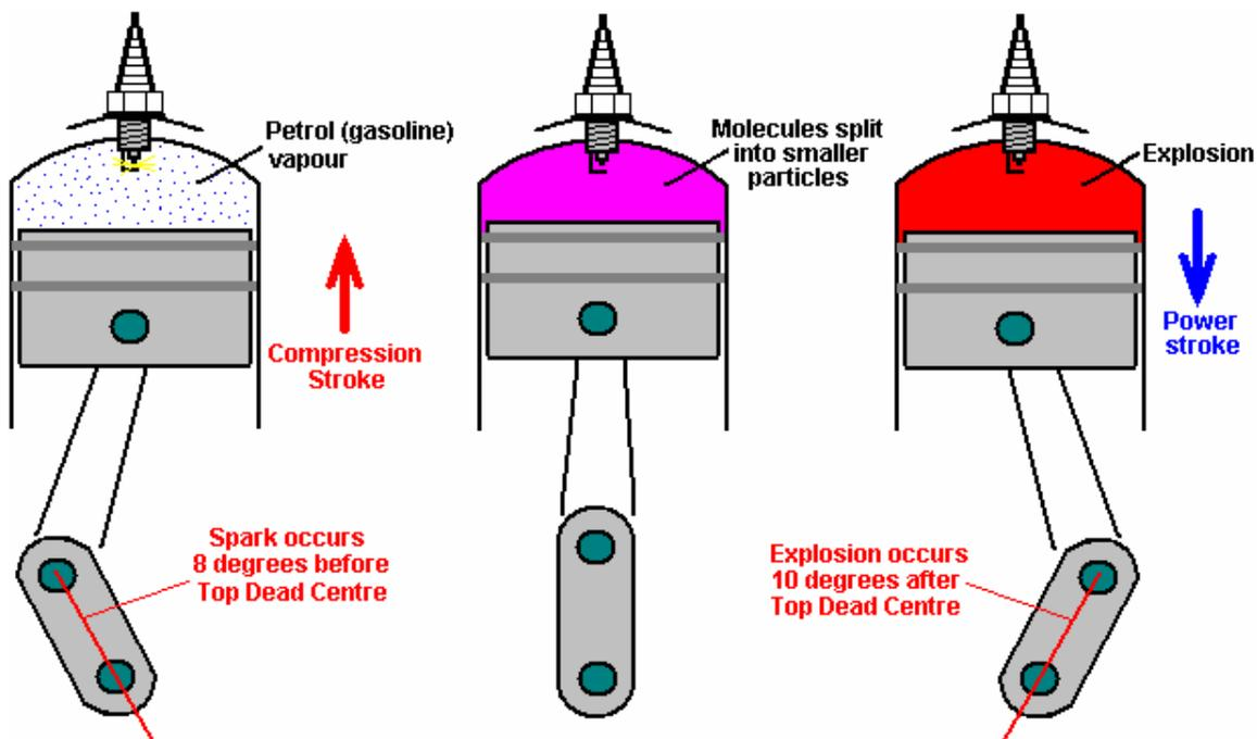
Because of the delay needed for the conversion of the hydrocarbon molecules to smaller particles, the spark is arranged to occur before the Top Dead Centre point. While the molecules are splitting up, the piston passes its highest point and the crankshaft is some degrees **past** Top Dead Centre before the driving pressure is placed on the head of the piston. This driving force then reinforces the clockwise rotation of the crankshaft shown in the diagram above and the motor runs smoothly.
