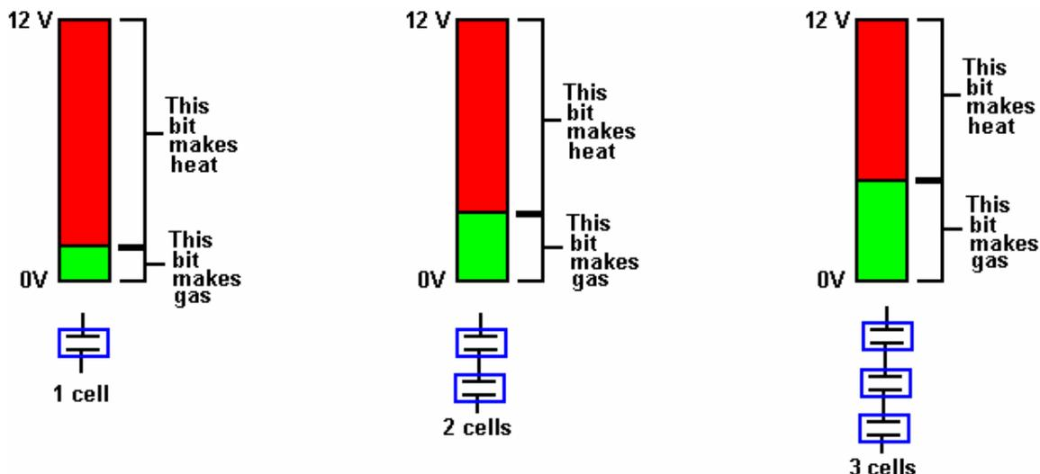
The best electrode material for the plates is 316L-grade stainless steel. It is hard to believe, but there is a voltage drop across the plate, which makes it necessary to apply about 2 volts to the plates on each side of the cell. So, if you are running off 12 volts, then six cells in a row across the battery gives the maximum possible drive. With the engine running and providing almost 14 volts, seven cells gives the highest possible drive.
