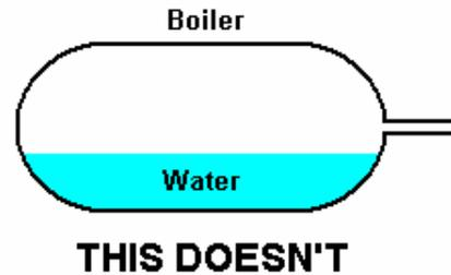
The power which drives the engine comes from burning the fuel. It does **not** come from the water, and in fact, if the engine were a Stirling engine, it would work perfectly well without any water being used at all. So, just to make sure this is clear, the power which drives a steam engine comes from burning a fossil fuel and the energy produced by that fuel burning could be used in various other ways which do not involve water at all.
