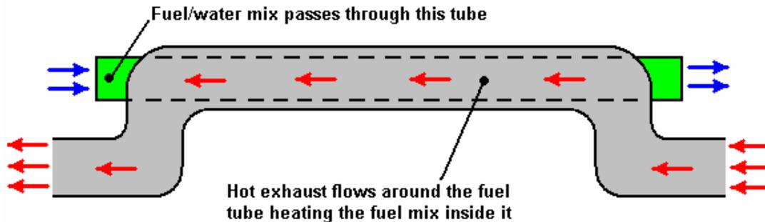
Here, the standard exhaust pipe is given a kink to move it clear of its normal run in order to allow an extra straight pipe of smaller diameter to be positioned inside it so that the hot exhaust gases are used to heat the incoming fuel flow. This is a useful energy gain as it uses some of the waste heat, raising the overall efficiency of the engine very considerably.
