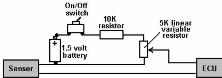
The circuit shown here allows a voltage anywhere from zero to 0.5 volts to be added to the oxygen sensor signal. This must **not** be done unless a booster is running. Using it without a booster is liable to lead to engine overheating and possible valve damage. This, of course, applies to the previous oxygen sensor signal adjusting circuit as well.
