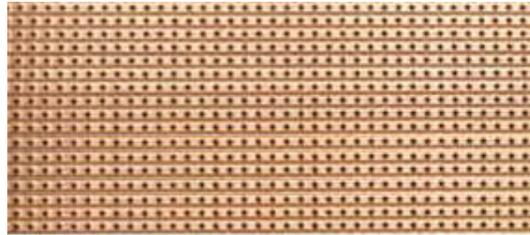
Strip-board (often called "Veroboard"), has copper strips attached to one side of the board. The copper strips can be broken where it is convenient for building the circuit. Component leads are cut to length, cleaned, inserted from the side of the board which does not have the copper strips, and the leads attached to the copper strips using a solder joint. Soldering is not a difficult skill to learn and the method is described later in this document.
