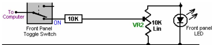
By moving the slider contact on the preset resistor “VR2”, any output voltage can be fed to the fuel computer. This voltage can be anything from the whole of the voltage across the LED, down to almost zero volts. We will use VR2 to adjust the output voltage when we are setting the circuit up for use. In this circuit, VR2 is acting as a
