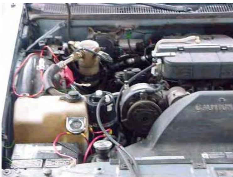
The unit draws only 15 amps which is easily handled by the existing alternator. The construction uses ABS plastic with Sodium Hydroxide ("Red Devil" lye, 1 teaspoon to 8 litres of distilled water) and the gas-mix is fed directly into the air intake filter of the car engine. The electrodes are stainless steel with the negative electrode forming a cylinder around the positive electrode:
