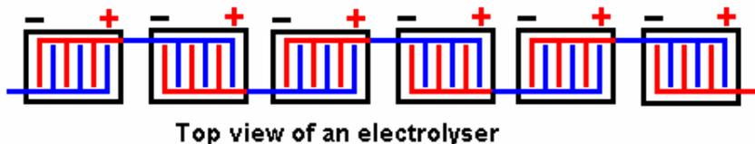
Here the plus side of each cell is connected to the minus side of the next cell to provide a set of six interconnected cells acting in series. The current flowing through the electrolyser goes through each cell in turn and so each cell receives exactly the same current as the other cells. This is the same sort of arrangement as using six Archie Blue style cells in a daisy-chain. To reduce the physical size of the unit, it would be possible to construct the electrolyser as shown here:
