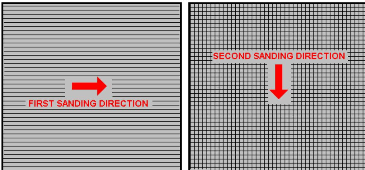
Bob uses a 6-inch x 48-inch belt sander which is great for preparing the plates and he uses it all the time now with 60 or 80 grit. Always wear rubber gloves when handling the plates to avoid getting finger marks on the plates. Wearing these gloves is very important as the plates must be kept as clean and as grease-free as possible, ready for the next stages of their preparation.
