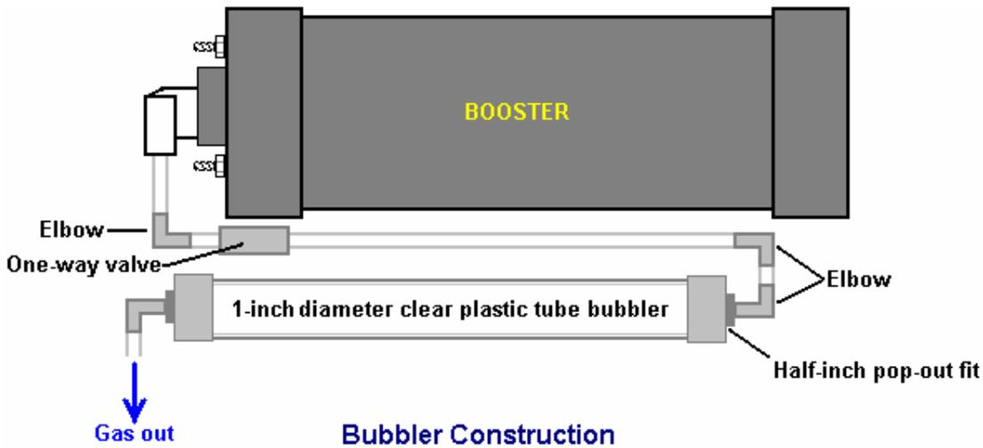
The elbows at the ends of the one-inch diameter bubbler tube have their threads coated with silicone before being pushed into place. This allows both of them to act as pressure-relief pop-out fittings in the unlikely event of the gas being ignited. This is an added safety feature of the design. However, it should be realised that the very high ignition rate of hydroxy gas creates a shock-wave which moves so fast that no pop-off fitting will ever be fast enough to rob it of its power.
