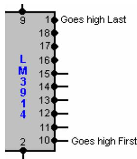
If the input voltage coming from the oxygen sensor is low, then all of these ten outputs will have low voltages on them. When the input voltage rises a little, the voltage on Pin 10 suddenly rises to a high value, while the other output pins still have low voltages.
