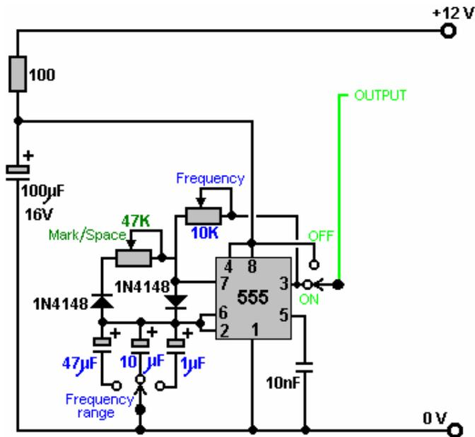
Which just has one additional switch to allow the output to be shipped and the 12-volt supply line to be fed instead. The reason for this is that this part of the circuit is used to switch On and Off an identical circuit. This is called "gating" and is explained in Chapter 12 which is an electronics tutorial.
