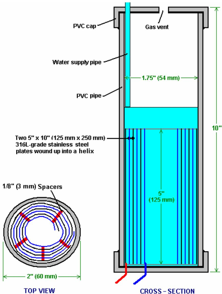
As the spring metal pushes outwards in an attempt to straighten up again, spacers are used to keep them evenly separated along their whole length by inserting 1/8" thick vertical spacer strips. The connections to the plates were made by drilling a hole in the corner of the plate, splitting the stranded wire, inserting the wire through the hole from both sides, turning it back on itself and making a wire-to-wire solder joint on both sides of the steel. The joint is then insulated with silicone.
