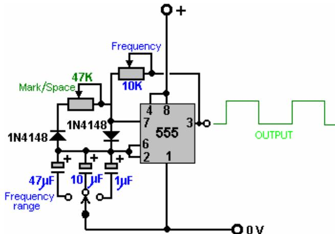
The capacitors shown here are unusually large because this particular circuit is intended to run relatively slowly. In the almost identical section of the circuit which follows this one, the capacitors are very much smaller which causes the switching rate to be very much higher. Anyway, the complete version of this section of the circuit is:
