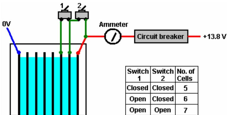
Here, the arrangement is very simple with two switches allowing one or two additional cells to be added in.
