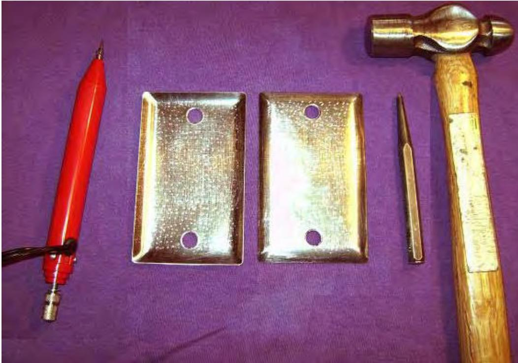
Shown above are typical hand tools used to create the indentations on the plates. The active plate surfaces – that is, the surfaces which are 1.6 mm apart – are indented as well as being sanded.
