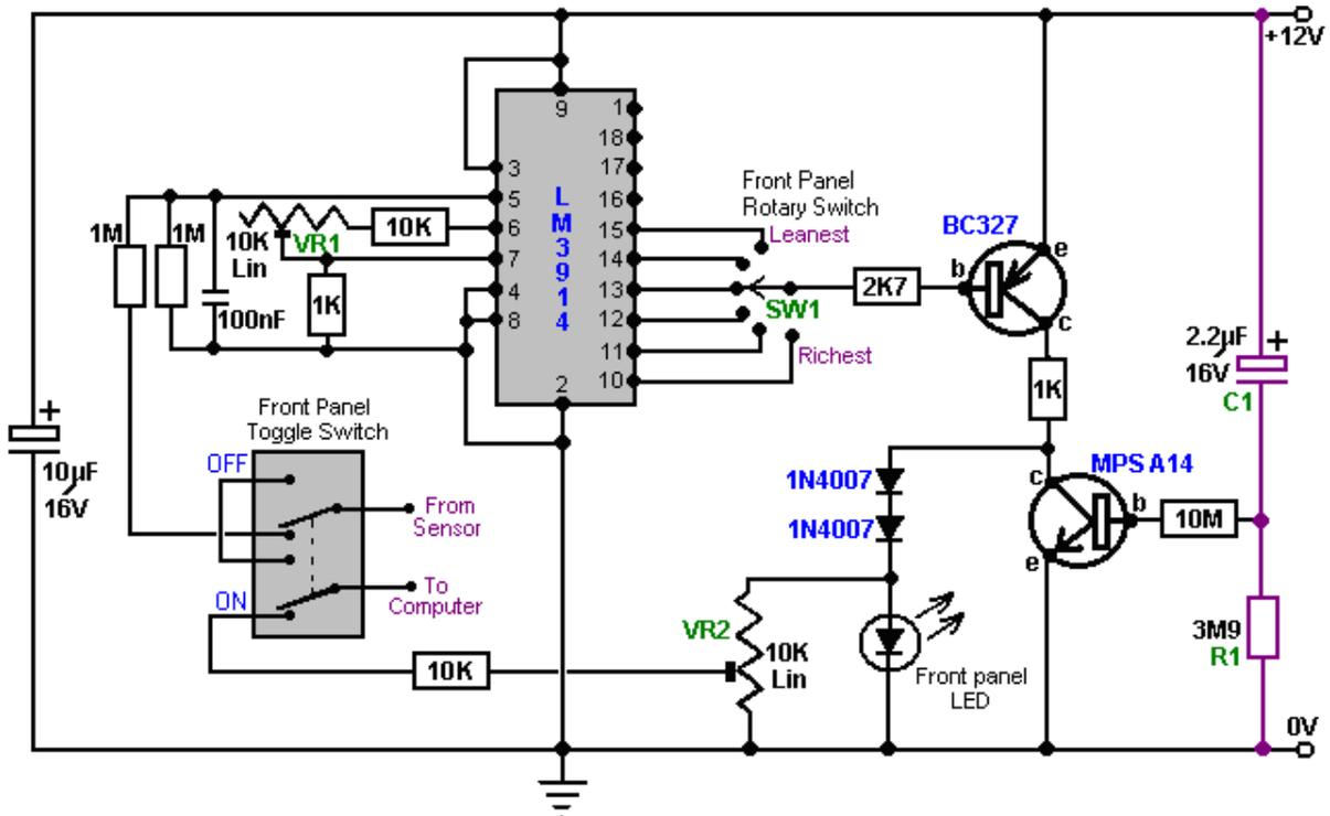
Electronic circuits are normally “read” from left to right, so we will look at this circuit that way. The first component is the 10 microfarad, 16 volt electrolytic capacitor. This is put there to help iron out any little variations in the voltage supply, caused by surges in the current drawn by the circuit when it switches from one state to another.
