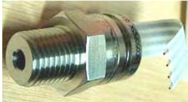
The pressure switch just mounts on one of the end caps of the pressure tank and the switch electrical connection is placed between the relay and the electrolyser. If the gas pressure hits its maximum value of 30 psi. then the switch opens, stopping electrolysis until the pressure drops again:
