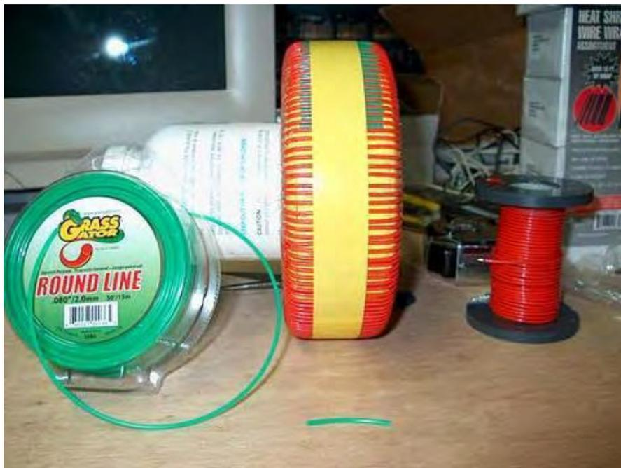
As you can see here, Bob uses short lengths of plastic trimmer cable as spacers for the outside of the toroid, though the picture above has been taken to show what a partially prepared secondary winding looks like when its windings are being moved into very accurate positions.
