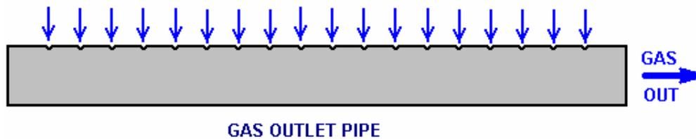
This arrangement works well as it allows large volume gas flow out of the cell and yet makes it difficult for any splashes of electrolyte to make it into the pipe.
