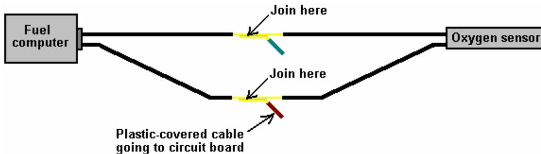
**Step 1: Remove a small piece of insulation and join the new cable to the original wire without cutting the original wire**
