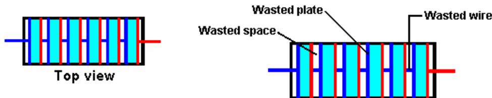
In this arrangement, the individual cells have just one positive plate and one negative plate. The plates slot into the sides of the housing so that the electrolyte is trapped between the plates and an air gap is formed between the plus plate of one cell and the minus plate of the next cell.
