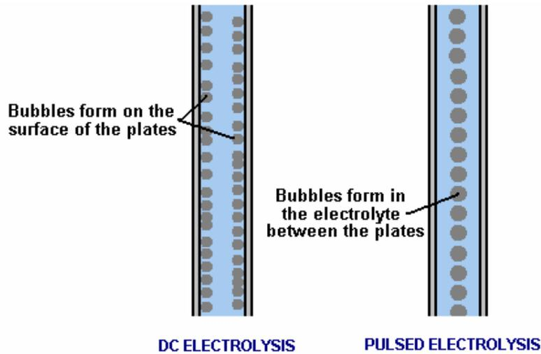
With straight DC-electrolysis, the bubbles of hydroxy gas form on the face of the plates and break away, helped by the thousands of microscopic, sharp-peaked mountains created on the face of every plate by the two-direction scoring with sandpaper. With the pulsed technique, the hydroxy bubbles form in the electrolyte itself, between the plates and give the visual impression of the electrolyte boiling.
