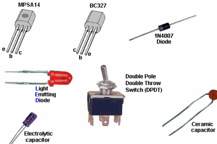
The MPSA14 and the BC327 devices are transistors. They each have a "Collector", a "Base" and an "Emitter" wire coming out of them. Please notice that the two packages are not identical, and take care that the right wire is placed in the correct hole in the strip-board before soldering it in place.
