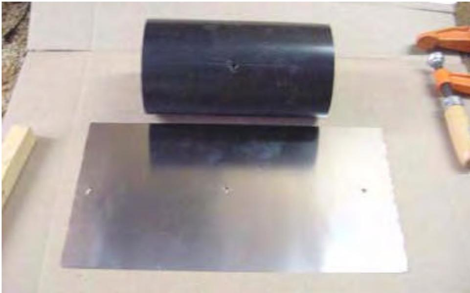
The shimstock holes need to be reamed to accept the capscrew.
