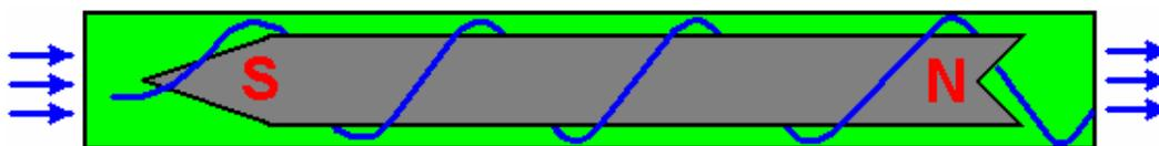
However, the magnetism of the solid rod, causes a most unusual effect and instead of the helical gas flow being as shown above, a highly uneven flow pattern is created. This causes the fuel flow to bunch up in the centre of the tube, generating a hot spot which creates quite unexpected results:
