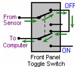
the connection from the oxygen sensor is passed straight through to the vehicle’s fuel computer, bypassing the circuitboard completely. This switch allows the whole circuit to be switched Off should you want to do this for any reason.
