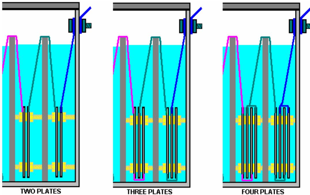
The electrolysis takes place in the gaps between the plates, so with two plates, there is just one area of electrolysis. With three plates, there are two inter-plate spaces and electrolysis takes place on both sides of the central plate in each compartment. With four plates, there are three inter-plates spaces and electrolysis takes place on both faces of the two inner plates in each compartment.
