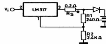
Fig. 8 Simple battery charger using LM317 voltage regulator
