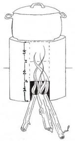
A short chimney above the fire forms a 'combustion chamber' where more gases can burn in the flames
