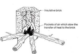
A smoky fire full of smouldering wood means that the fire is not hot enough to burn the gases being released from the wood.
