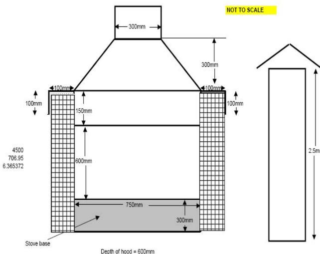
The *upes*i stove works best when thin pieces of very dry wood are regularly added to the stove. Where people are very short of fuel, they will conserve it carefully by burning it in this careful way. The dimensions of the smoke hood used in Tanzania are shown in Figure 5.
