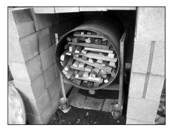
The loaded retort inside the kiln.
