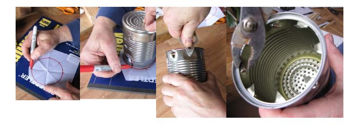
Step 4: Punch air inlet holes in the outer can
