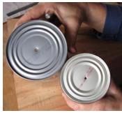
Step 2: Punch primary air feed holes in the bottom of the inner can Air will come up through the bottom of the small can to feed the fire. Take the nail and hammer and punch a large number of holes around the center hole in the bottom of the can. Make sure the entire bottom of the can is covered in holes about 2-3mm apart.
