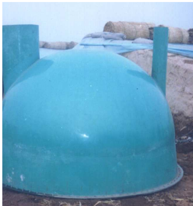
Figure 3: Glas fiber digester made in China (source: www.biogas.cn )
