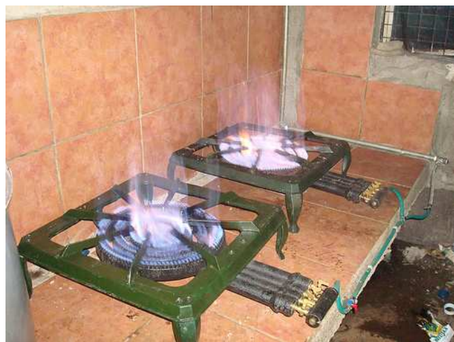
Figure 5. Biogas cooker at Gachoire Girls High School in Gachoire, Kenya (source: S. Blume, 2009).
